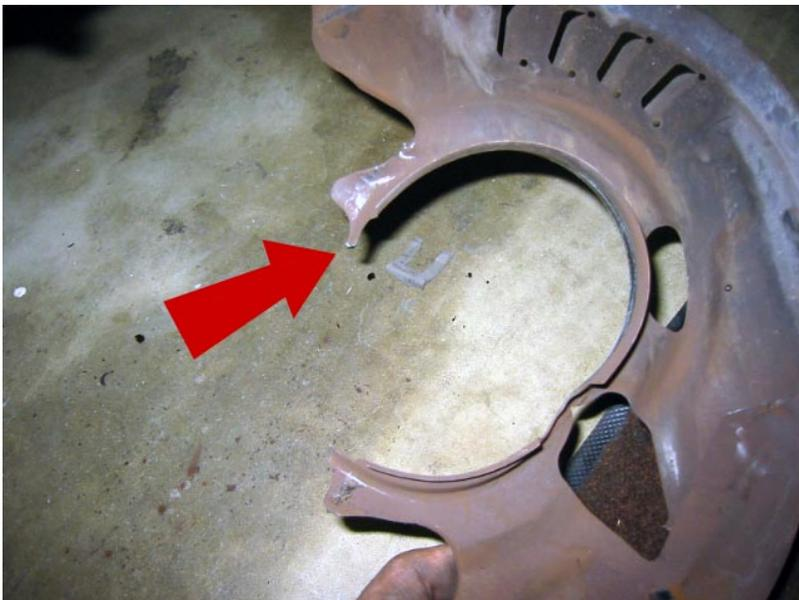
**Figure 2** – Cut factory dust shield at the front of the hub.
