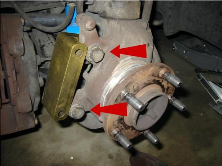
**Figure 4** – Bolt adapter to spindle using OE caliper hardware
