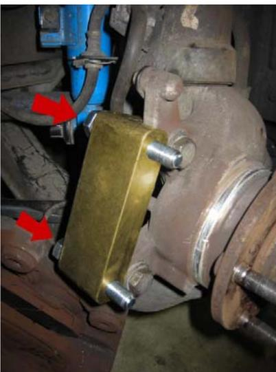
**Figure 5** – Use supplied lockwashers and long caliper bolts
