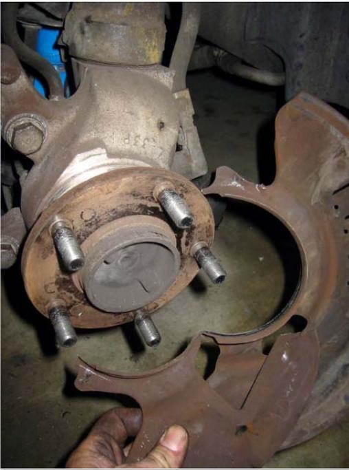
**Figure 3** – Removing factory dust shield.
