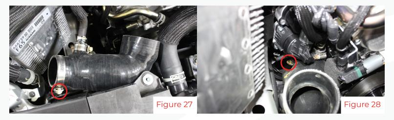
15. Position the passenger airbox over the silicone and align the stanchion over the grommet. Clock the silicone until the airbox and silicone are properly aligned. Tighten the clamp on the turbo inlet(fig 29).
