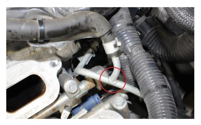
20. Due to the design of the fuel rails, the passenger rail needs to be remove first. Remove the two nuts and two bolts holding the passenger side fuel rail to the cylinder head. Work the rail free and remove it as shown below.
