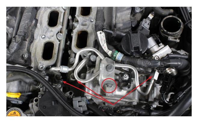
18. Remove the two bracket bolts holding the hard pipe on the back of the head to create more room to slide the fuel rails out.
