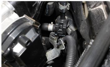
14. Disconnect the two throttle body connectors, the EVAP connector and the hose from the valve cover as shown below.
