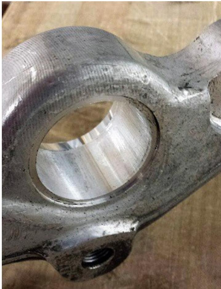
Installing the bushings is the reverse of removing the old ones. Use the 1 1/8 inch socket as a driver after starting the new bushings. Press them in until the flat side is nearly flush with the bushing. It may be necessary to take the arm off the press to visually inspect progress.
