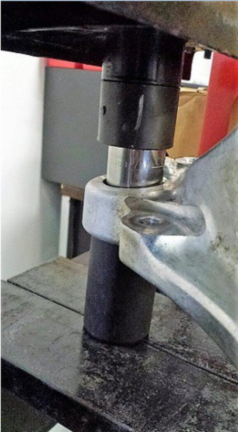
Press out stock bushing using appropriate bushing press and driver. As shown, we used a 1 1/8 inch socket as the driver. Also keep the flat side of the arm facing down.
