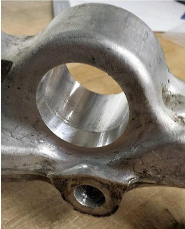
The chamfered side of the bore should be facing up when installing the bushings. Here is what the chamfered side looks like:
