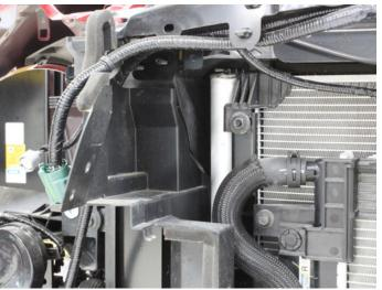
**22.** Remove the plastic air duct.
