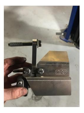
14. Go ahead and also connect the other end of the clutch line to the slave cylinder using the banjo bolt and crush washers included with the line. With the line already connected, mount the slave cylinder assembly to the bulge in the bellhousing where the starter lives using the two longer flanged M10 bolts. It can help to have the fork adjustment bolt threaded in fully so there is as much room as possible to maneuver it in.
