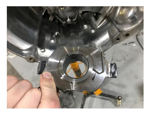
9. Now slide the throw out bearing carrier onto the center guide shaft and seat the fingers of the fork on the wings of the carrier, making sure to slip the ends of the spring into the grooves on the back of the fingers on the fork and clip the two parts together. (it should look like this when it's all together on the inside)
