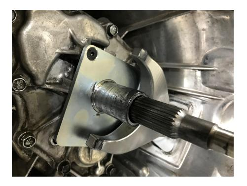
8. Grease the bottom of the two 'wings' of the throw out bearing carrier and install the retaining spring for the fork onto the bottom of the carrier.
