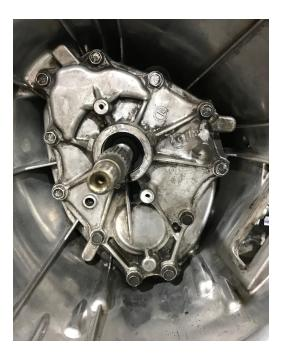
3. Remove the two 12MM head M8 bolts at the 4 and 5 O'clock positions when you are facing the input shaft of the transmission. Mount the bent steel base plate and the central guide column loosely using the countersunk M6 bolts using some blue or orange threadlocker. Thread in the new M8 bolts also using some blue or orange threadlocker and tighten all 4 bolts now securing the base plate to the transmission.
