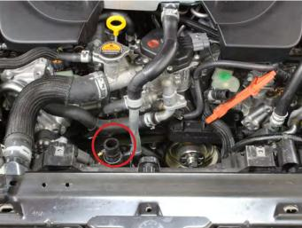
**08.** Set the new Red Alpha Coolant Expansion Tank in place and connect the smaller radiator side hose first. Once connected, set the coolant expansion tank in place and align the larger intercooler hose. Once in place, reinstall the OEM clamp or tighten the supplied #10 clamp. Use an extension and 5/16" socket to access the #10 clamp from the passenger side air box area.
