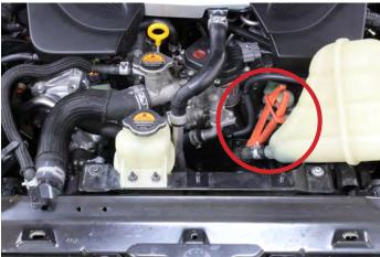
**04.** Remove the clamp and carefully slide the hose off. Do so as you till the expansion tank backwards to avoid coolant loss. There will be some coolant spill, just use clean water to rinse the excess coolant down and it will dry on its own. Save the coolant in the expansion tank and it can be reused.
