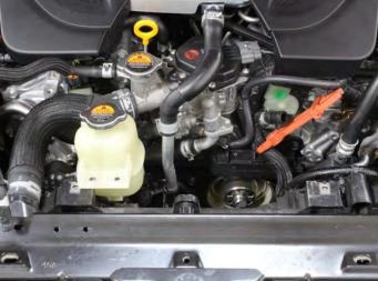
**06.** With the bracket removed and the expansion tank loose, it will be easier to remove clamp and hose from the expansion tank. Drain the coolant from the tank. You can do so by drawing it out the top or by draining from the OEM drain under the right front bumper area.
