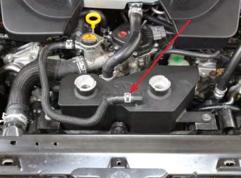
**10.** Reinstall the cowl cover / air duct and fill the coolant expansion tanks. Fill both tanks half way up. The tank measures 4" from the bottom of the tank to the bottom of the filler neck. Use a stick and measure out 2" from the end. Use this as a gauge to measure the fluid level. Run the car for a minutes and recheck the fluid level. Drive the vehicle for a full drive cycle and let cool completely. Recheck again once at ambient temperature, adjust as necessary.
