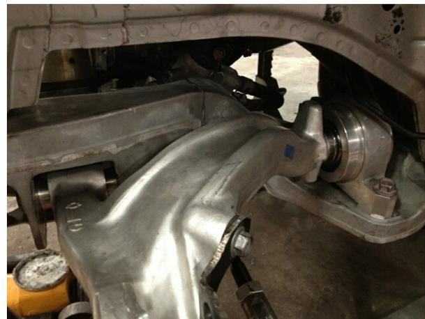
5. Measure the inner diameter of the bushings and the stud. The stud should be at least 0.001 inch thicker than the inner diameter of the bushing bore. If it isn't, knurl the stud some, and you can also add bearing assembly compound.
