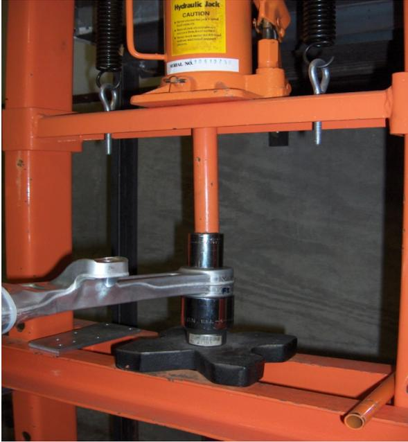
1. Press out the stock bushing using an appropriate bushing press and driver. For reference, we used a 2 in. ID Steel pipe and a 32mm socket.
