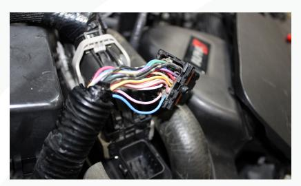
34) Cut the wire about 1.5" away from the connector. This is a good spot to allow the harness to flex slightly when its in its connected position. Strip both ends to prepare the crimp.
