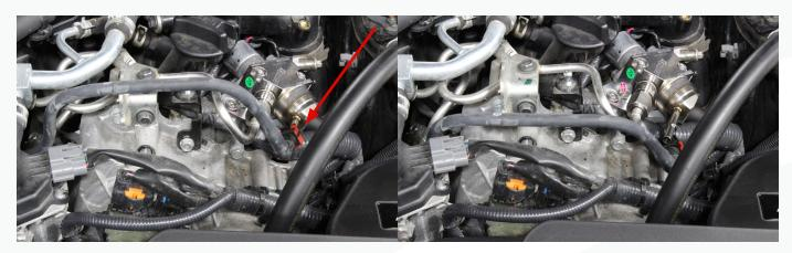
9) On the right side of the engine, disconnect the low-pressure fuel line from the bracket on the engine as shown.
