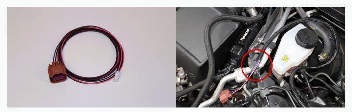
46) Carefully feed the harness over to the CAN module while staying clear of the wiper mechanism and plug it into the CAN module.
