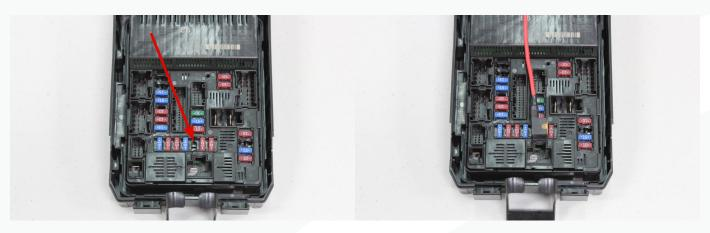
26) Route the harness around the battery area. Connect the red wire of the wire harness to the fuse tap and route the wire along the factory harness leading out of the bottom of the IPDM housing.
