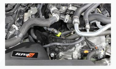
16) Route the hose as shown to the forward most fitting on the flex fuel sensor and tighten the fitting. The new fuel line will route under the A/C hose along the front of the engine.
