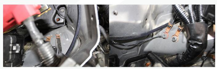
41) Locate the CAN-bus module and dual lock. Cut the dual lock into (2) 2" sections. Clean off the back of the module and mount one section on the lower half of the back.
