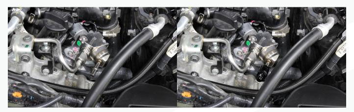
18) Locate the remaining supplied fuel hose. This hose can be installed in both directions to offer options for different HPFPs. The hose shown is installed on an AMS HPFP, so the 180-degree fitting is attached to the HPFP and the 150-degree fitting is installed on the flex fuel sensor. The fuel hose can be routed over or under the A/C hose depending on the configuration.
