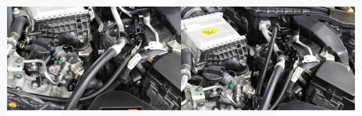
19) Alternately, if using the AMS Big Bore HPFP, the inlet fitting on the pump is a male -6AN. Attach the 180-degree fitting to the flex fuel sensor and the 150-degree fitting to the fuel pump.
