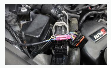
37) Using some electrical tape, start at the loom and rewrap the harness towards the connector.
