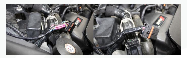
38) Reassemble the connector and re-secure the loom to the connector with a small zip tie.
