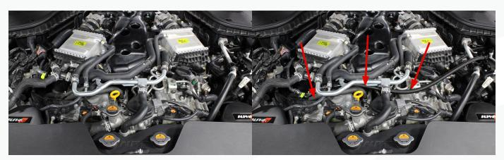
15) Reattach the fuel line to the new bracket as shown on the right side of the engine. Make sure the OEM fuel line is properly clipped into the plastic bracket.
