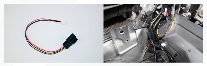
44) Neatly bundle up the slack in the power wire harness and secure it with a zip tie. Tuck the harness away under the battery tray.
