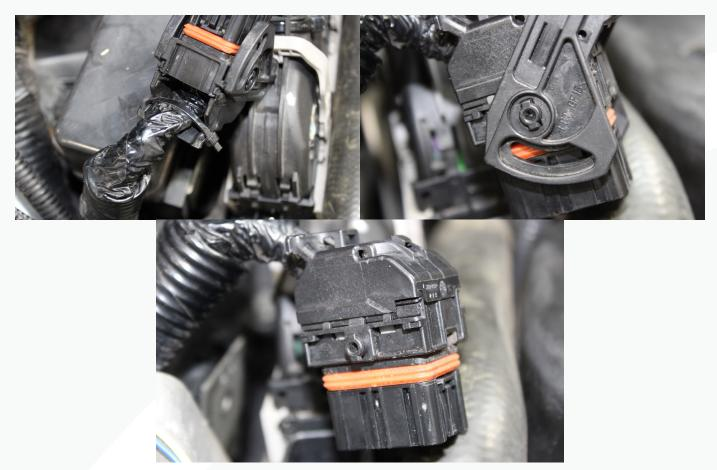
31) There are two small lock tabs at the front of the connector. With a small screwdriver, release the tabs one by one while pushing the connector cover forward.
