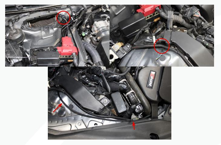
29) Disconnect the smaller black ECU connector by pushing the tab down and rotating the lock.
