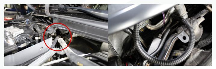
47) Pull slack from the harness to the brake reservoir and secure it to the ac line with a zip tie.
