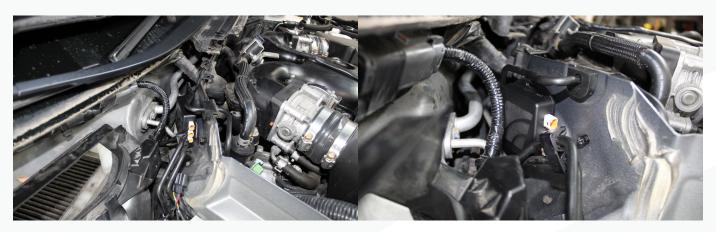
43) Locate the short jumper harness and plug the white 4 pin connector into the box. Then plug in the black 4 pin connector into the main harness.
