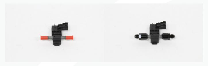
4) Locate the flex fuel sensor mounting bracket and strap. Use the two supplied M5 button head bolts and attach the flex fuel sensor to the mount as shown.
