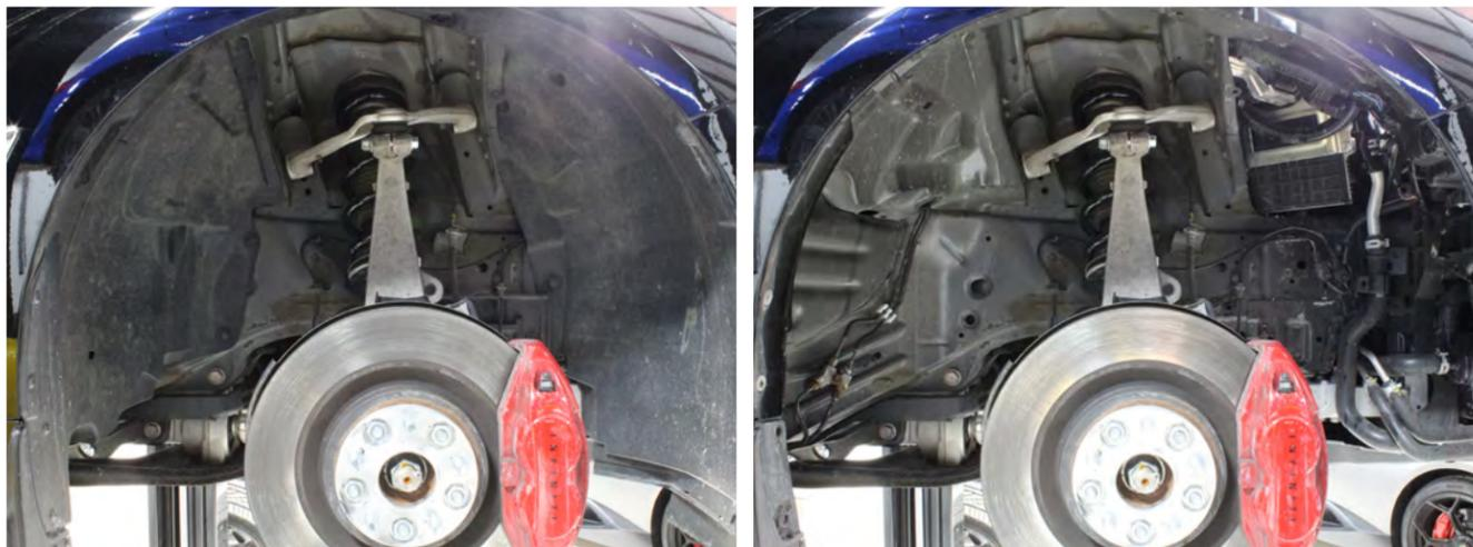
4. On the inside of the fender, there are several holes in the rear leading into the door jamb area. Two of these holes will be used to mount the tank. These holes are covered by a black textured round sticker that can be seen with the right / passenger door fully open. Locate the two holes shown in the pictures and carefully remove these stickers.
