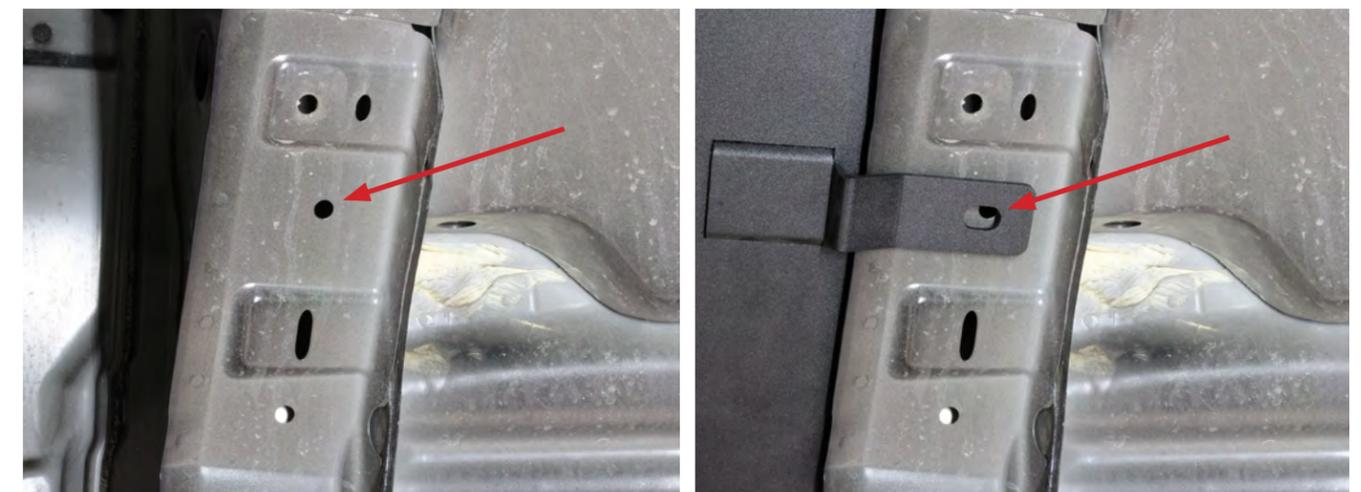
6. Use a 7/16" drill bit to open the hole up. Next, locate and install the supplied stainless steel M8 rivet nut. This rivet nut requires a special tool available online and at most tool retail suppliers. We have provided a link and information below for a tool we use here in house, but there are many types available to choose from..
