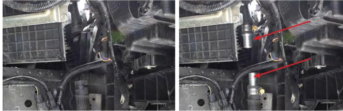
12. Next, route the water tank inlet hose as shown. Start by connecting the supplied hose and #10 hose clamp to the bottom inlet fitting on the water tank. Route the hose up the tank following the wheel well. The hose will run along the panel seam, then to the left of the head light and connect to the vertical hose you installed a billet fitting in step #11. Determine the hose length needed and cut it to length. Use a #10 hose clamp to finish the connection.
