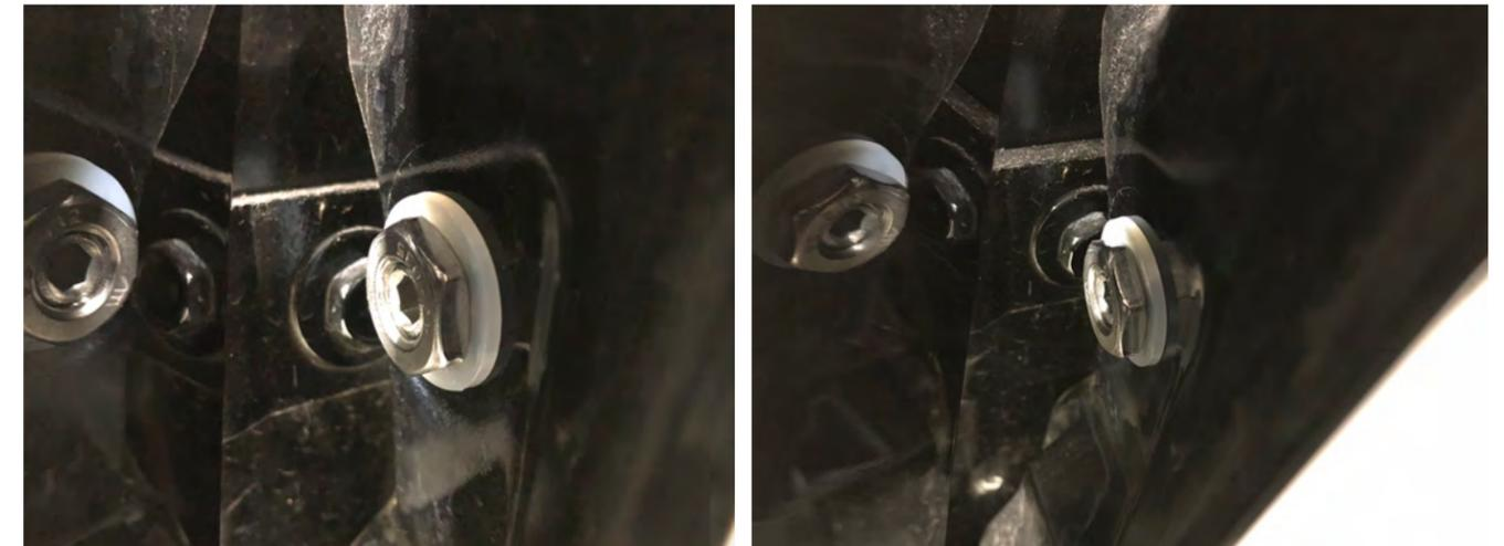
10. Drain the intercooler cooling system from the factory drain at the bottom of the right / passenger's front bumper area. Save the coolant if you wish to reuse. Once drained, remove the metal pipe and bracket shown. This pipe will not be reused.
