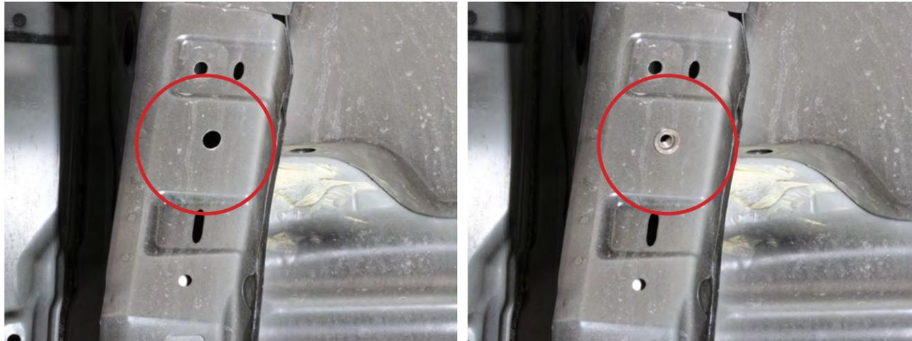
7. Once the rivet nut is installed, install the tank and secure the front bracket with the M8 stainless bolt as shown. contaminants into fuel tank..
