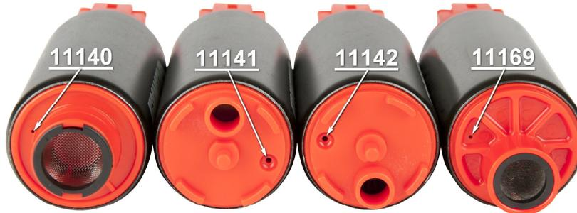
Please note the location of the vapor-purge port for your model Stealth 340, as illustrated above. During installation, be certain to check for and eliminate any blockage or restrictions to this port. Failure to do so may result in slow or no priming and may damage your 340 pump due to dry run.
