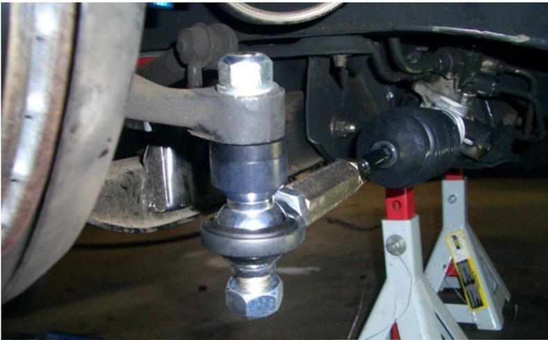
Install spacers. As pictured on left, the tie rod ends are installed with 1 adjustment spacer (flat ring spacer) and 1 misalignment spacer (large cone shaped spacer).
