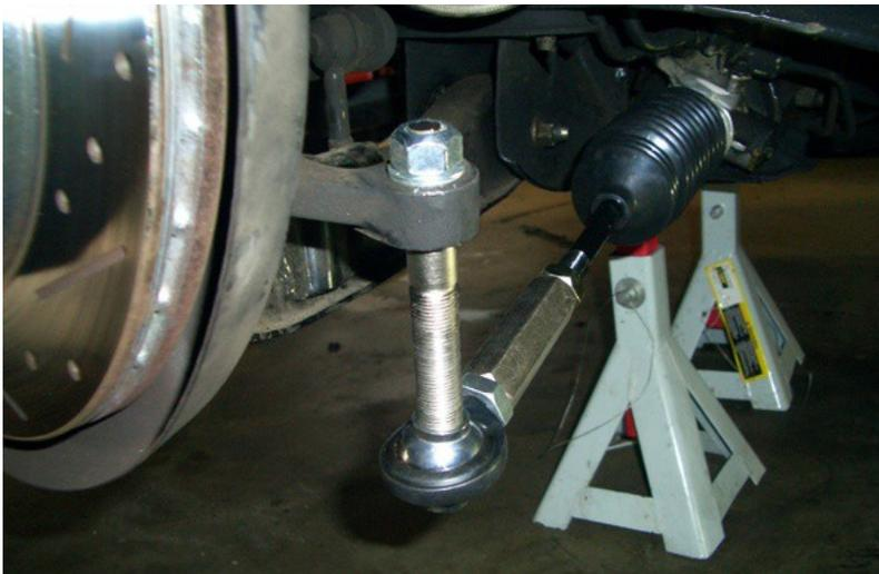
Use 2 supplied silver colored nuts, jam 2 nuts together to help hold the shank. **Torque nut on top of knuckle to 40 ft-lbs. DO NOT USE IMPACT GUN OR OVERTORQUE** otherwise strength of tie rod end will be severely compromised.
