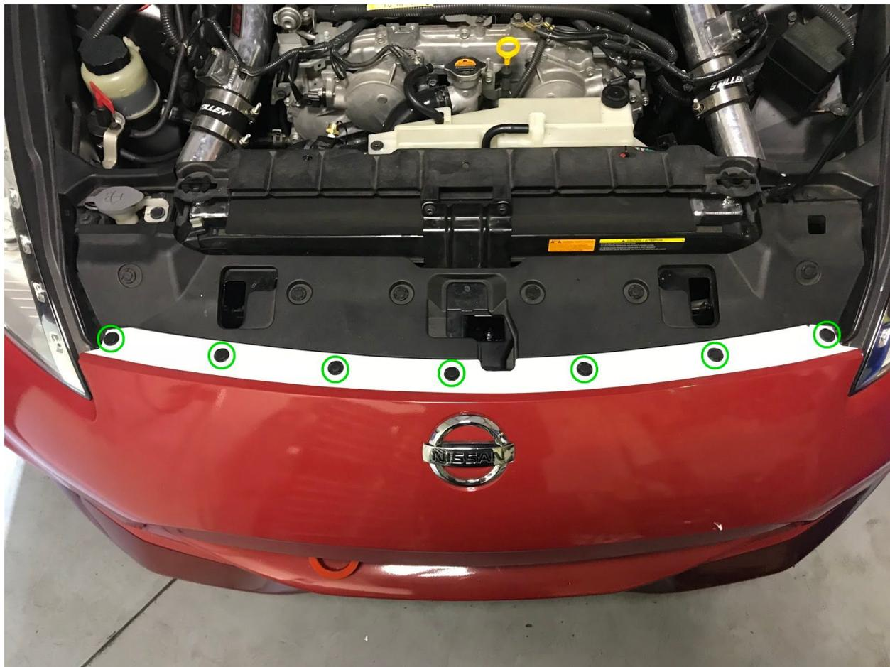
3. Lift the car and remove the ten 10mm bolts along the bottom of the bumper cover (yellow circles)
