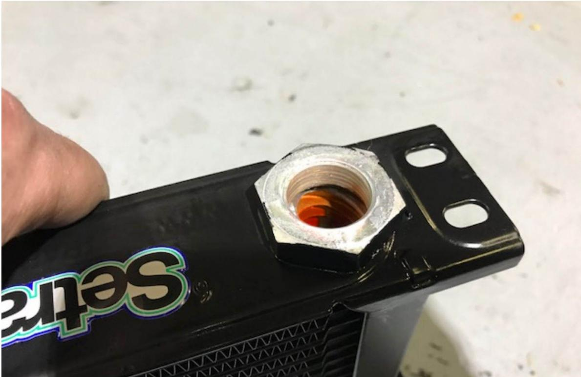
13. Apply a dab of fresh oil to the o-ring seal and thread the -6 AN to 22mm adapter fittings to the top of the cooler core and tighten them down. Take the 90 degree 3/8" push lock to -6AN fittings and thread them onto the top of the cooler loosely so they can be rotated later.
