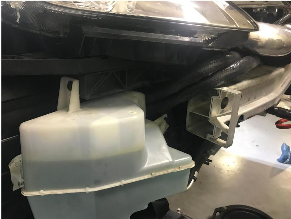
20. Slide the windshield washer reservoir neck back into place and apply a bit of pressure for it to “pop” back into the reservoir. Secure with the original pop clip.
