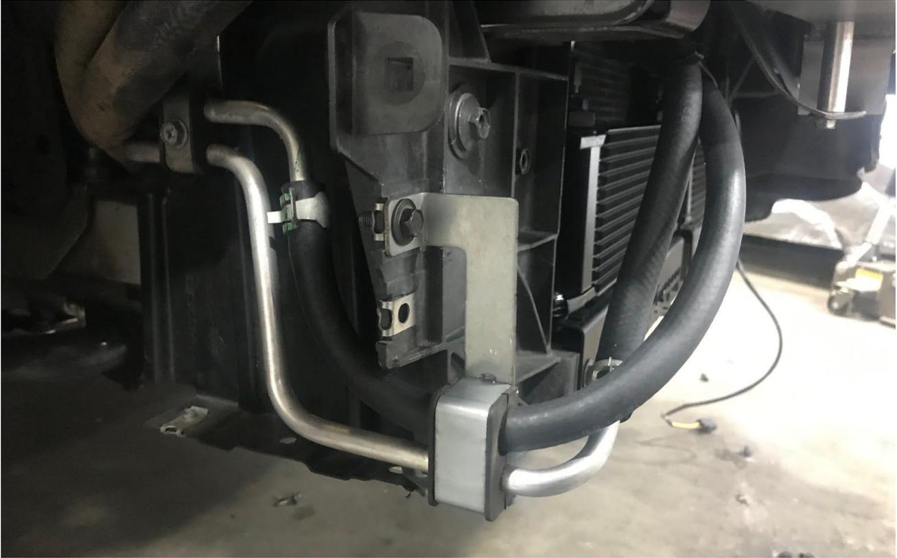
11. Attach the lower mounting bracket to the cooler core with the four of the supplied 10mm bolts, rubber washers and lock nuts. Use the 4 rubber washers in between the bracket and the cooler core to insulate the assembly.
