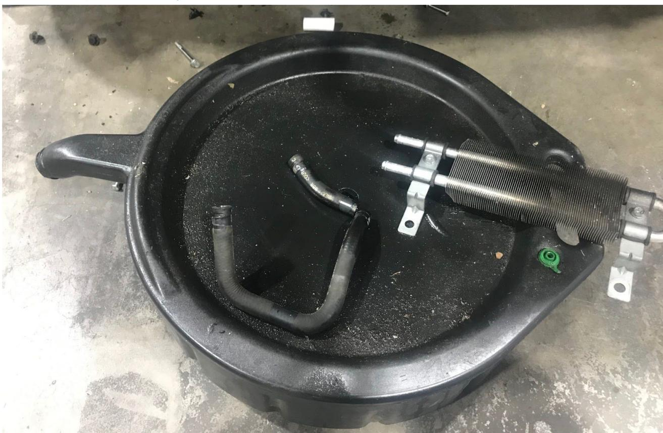
6. Remove the single 10mm bolt holding the power steering lines in place. Remove the clamps holding the short rubber line from the cooler and hardline on the car.
