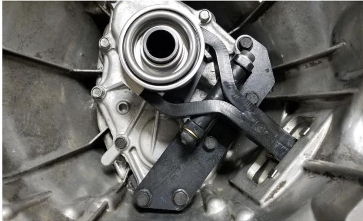
Tighten top and bottom 2 bolts on the the bracket finger tight while holding up of fork end slightly. (this centers the bracket) then finger tighten the other 3 bolts, TQ top and bottom bolts first to 20 ft-lbs and then tighten remaining bolts the same.\_Check fork operation, If throw out bearing does not move easily loosen 5 bolts on bracket and adjust holding slight pressure upwards on slave end of fork, tighten & recheck.
