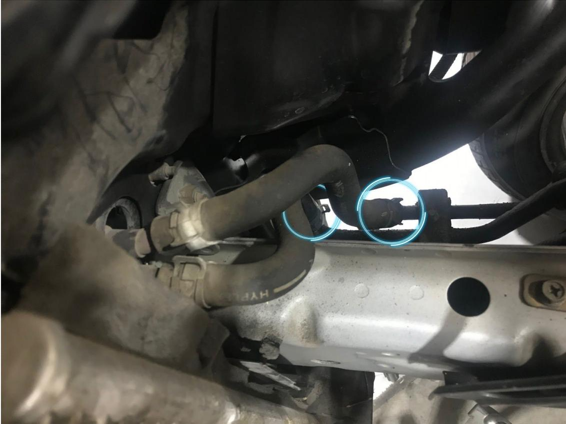
8. Remove the 10mm bolt securing the bracket that is holding the lines to the front core support, snip the zip tie holding it together and remove the bracket and rubber grommet as well as the two hard lines it was used to secure.
