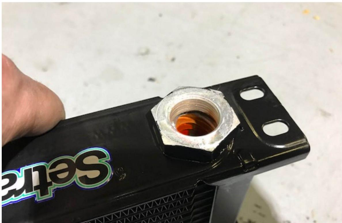
11. Apply a dab of fresh oil to the o-ring seal and thread the -6 AN to 22mm adapter fittings to the top of the cooler core and tighten them down.
