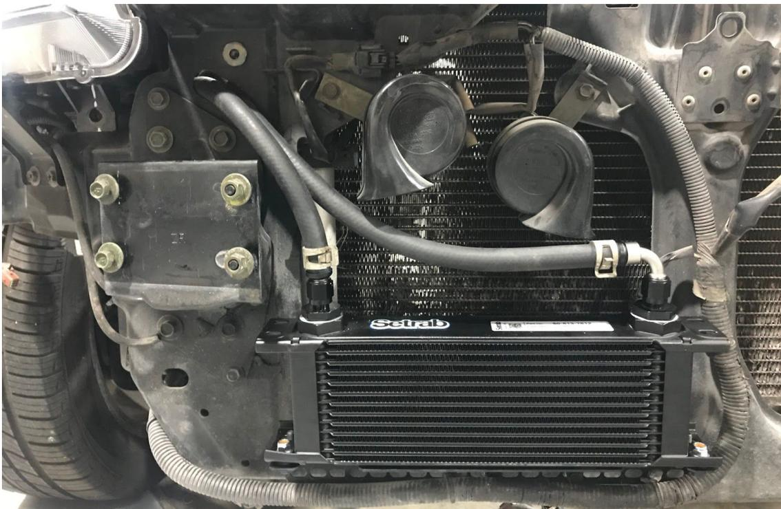
15. Refill the reservoir with fresh Nissan power steering fluid or a compatible replacement. Do not use store-brand power steering fluid; you can use Dexron ATF III or higher, if Nissan fluid is not available to you.
