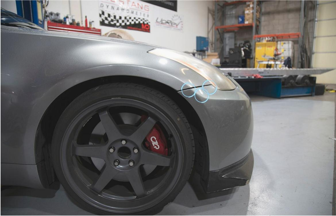
With the wheel turned inwards slightly, you can push the fender liner out of the way slightly and gain access to the two bolts going up into the fender and the one bolt going upward, mounting the bumper bracket to the headlight. All three are 10mm and may require the use of an extension.(Repeat for both sides)
