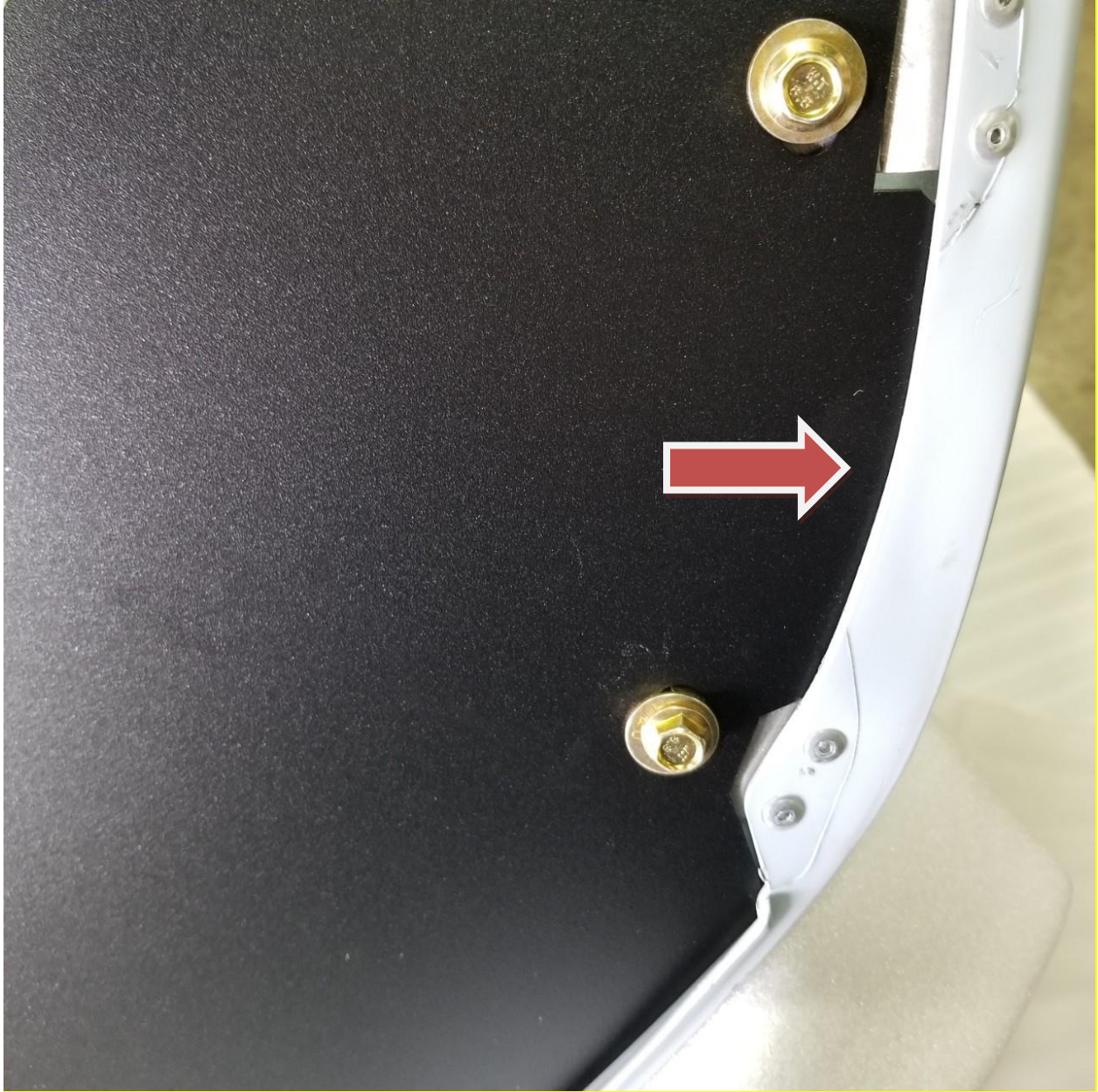
Install so that tab with red arrow goes above bumper lip.
