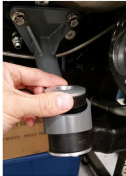
Place the thinner upper bushing with its aluminum washer onto the top of the mount and install the M10 x 70mm long flat head bolt – **it is very critical that you use the ARP lube on these particular bolts, since the bolts thread directly into aluminum.**
