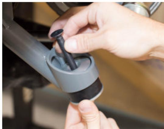
Torque the flat head bushing bolts to 30 ft-lbs (40 N-m) using the BDE supplied wrench to hold the bottom bushing locator while tightening. The small button should be oriented to the outside and straight with the mount arm's main tube (90° from the side of the engine) to allow it and the threaded stud to register into the slots in the chassis.
