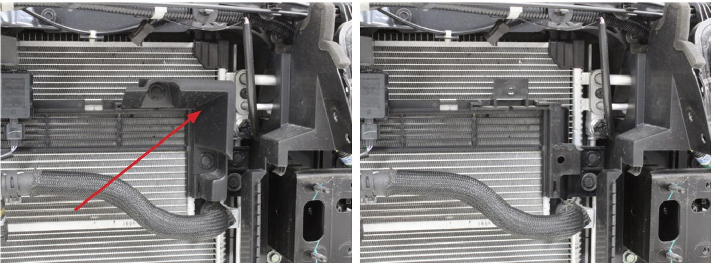
26. The radiator and A/C condenser needs to be moved towards the rear of the car. To do so, carefully use a pry bar and lift at the base of the rubber radiator mounts. **DO NOT LIFT ON THE PLASTIC END TANK OF THE RADIATOR!** You may also need to push the top of the radiator towards the rear of the car while lifting it upwards to clear the upper core support bracket. Once the rubber mounts are lifted out of the core support, push the assembly towards the rear.
