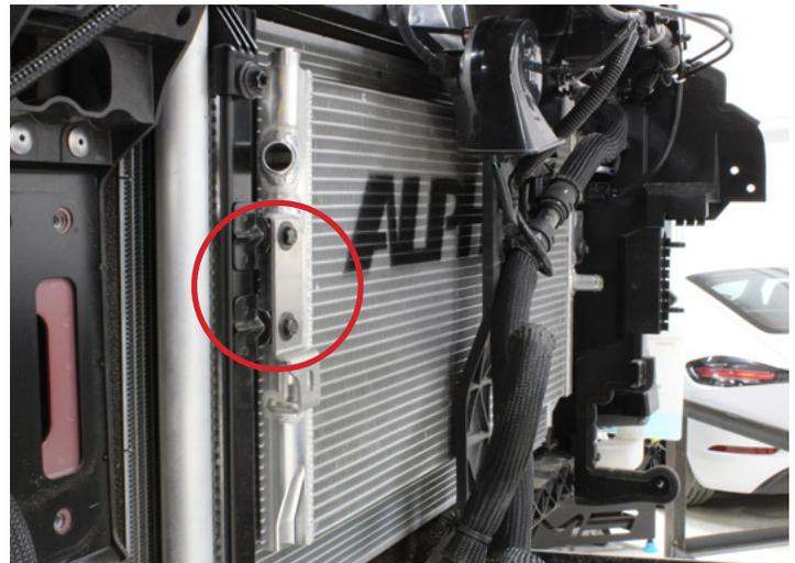
34. There is a union connection at the base of the heat exchanger on the right side. The clamps need to be rotated outwards from the heat exchanger to avoid damage to the heat exchanger.
