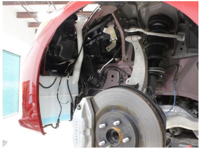
06. Disconnect the front LED running light harnesses on both sides. The connectors are located just below the headlights.
