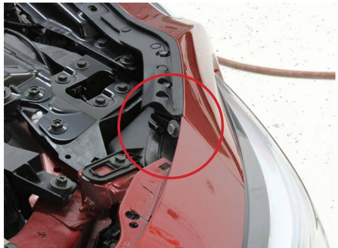
11. On the top of the bumper, remove the last two push pin clips.
