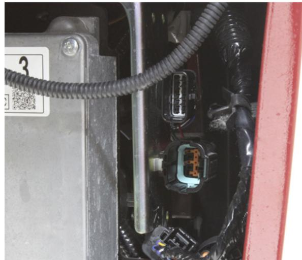
08. From the bottom of the car, disconnect both front fog lights.
