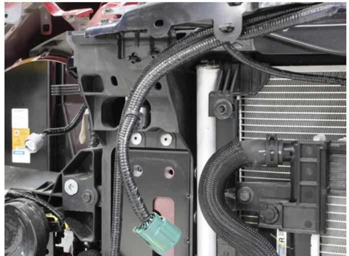
23. Remove the top radiator support plate. The Q60 and Q50 models vary slightly.
