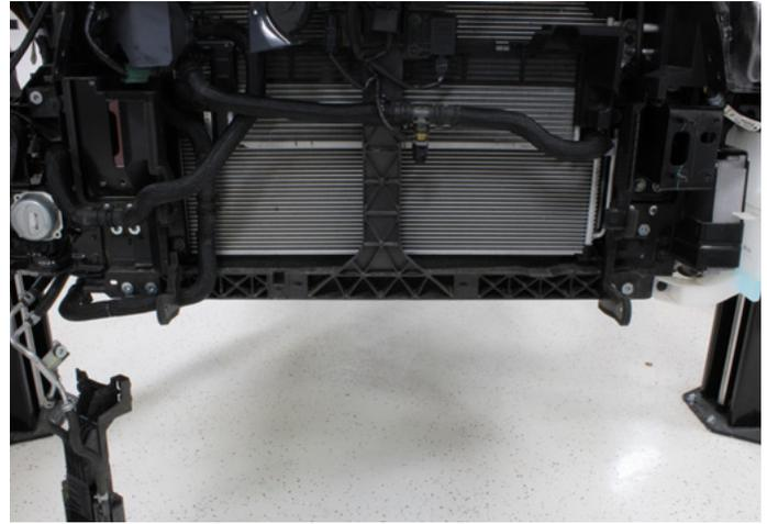
21. If you're Q60 or Q50 trim level is a Red Sport, you will need to unbolt the secondary water pump. Disconnect the electrical connector and unbolt the pump and bracket from the core support. You will not need to disconnect the hoses from the water pump. Allow the pump to hang.
