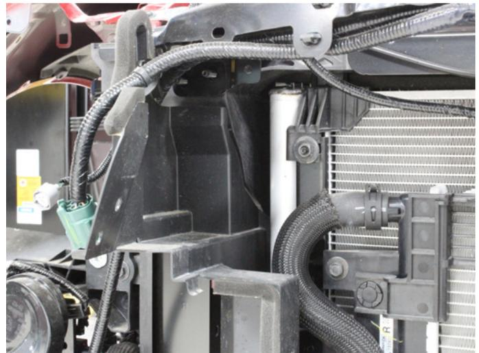
22. Remove the plastic air duct.
