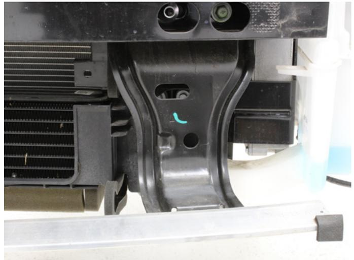
16. Remove the crash beam. The Q60 has a louvered lower section controlling air to the engine oil cooler. Make sure to disconnect the harness on the lower left side of the crash beam and remove as an assembly. Also make sure the outside temperature sensor on the Q60 is disconnected since it is attached to the crash beam.
