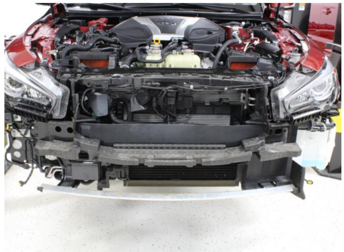
13. Remove the foam crash beam insert along with any plastic trim panels that overhang the crash beam.
