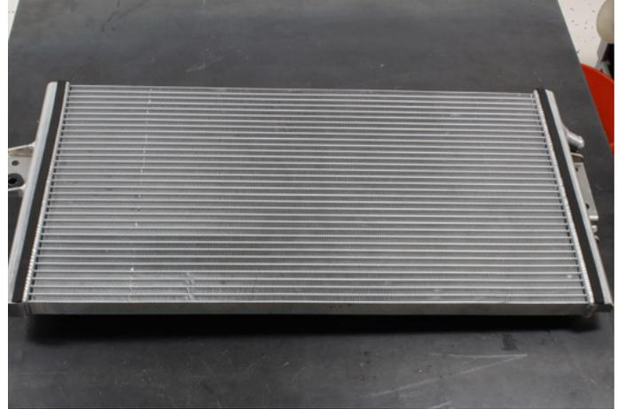
31. Carefully install the Infiniti Red Alpha heat exchanger in the car. Use the factory bolts and mount the heat exchanger loosely.
