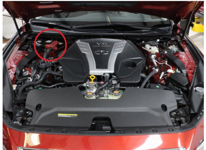
02. Remove the engine bay trim panels that run along the front fenders. These can be difficult to remove. Start at either end, pull straight upwards releasing the clips underneath. While pulling upwards, wiggle the panel around to try and release the clips. Plastic panel trim tools can also be used to get under the panel to pry upwards as well.
