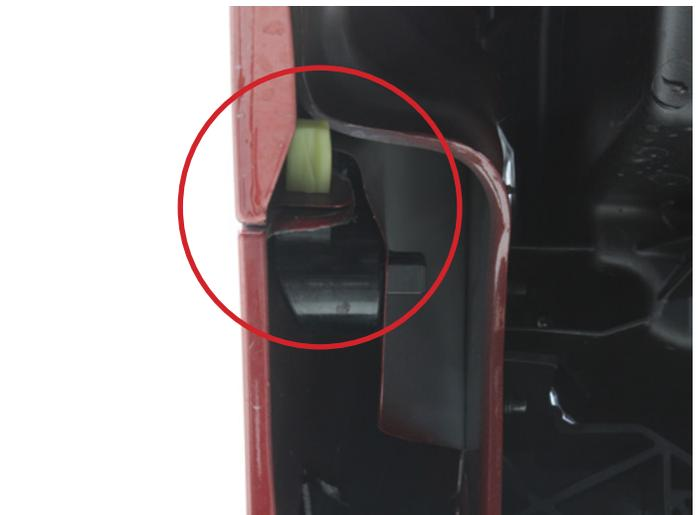
10. Just above the headlights where the top of the bumper and the fender meet, there is a bolt and retainer plate holding the two together. Remove the hardware shown.
