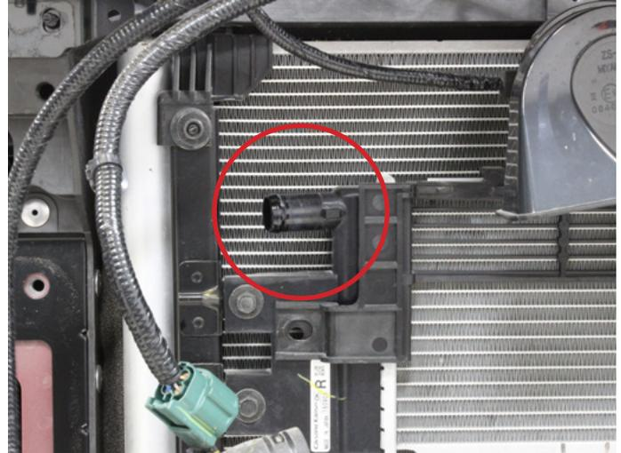
28. Carefully remove the three bolts holding the factory heat exchanger in place. Carefully remove the heat exchanger by sliding it out the right side of the car. There is a plastic guard still attached to the heat exchanger, remove if necessary.
