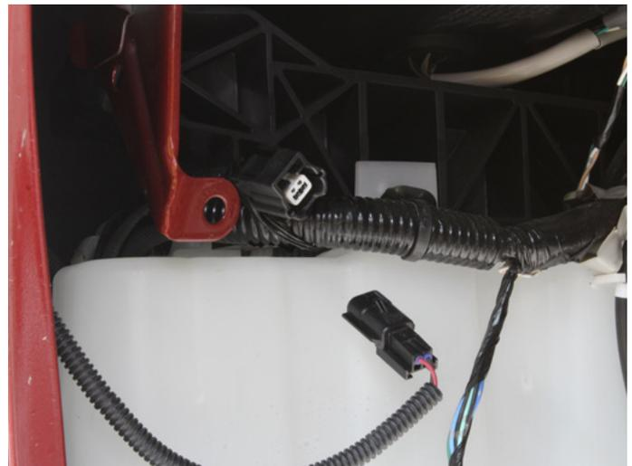
07. Inside the passanger side wheel well just behind the bumper, locate and disconnect the two connectors for the parking sensors and front camera.
