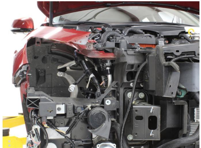
18. Remove the right side crash beam mount. These are specific bolts holding the mount in place. They are 13mm hex head bolts that look similar to the 12mm hex head crash beam bolts. Make sure not to mix them up during reinstallation.
