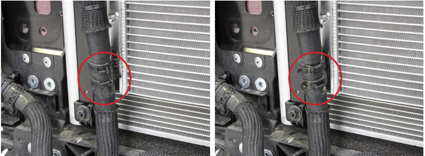
35. On the Q60 and Q50 Red Sport models, check the clearance of the secondary intercooler coolant pump inlet hose to the Infiniti Red Alpha heat exchanger. During reassembly, this area can be adjusted in two ways. First would be to bend the bracket slightly rotating the intercooler pump outwards and the hose away from the heat exchanger. The second would be to disconnect the pump inlet hose and using hose cutters, trim a small piece off making the hose slightly shorter.
