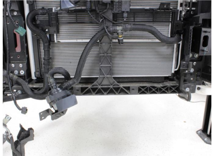
27. Disconnect the inlet and outlet hose on the factory heat exchanger. Make sure to have a drain pan under the disconnection point to collect coolant that still remains in the system.
