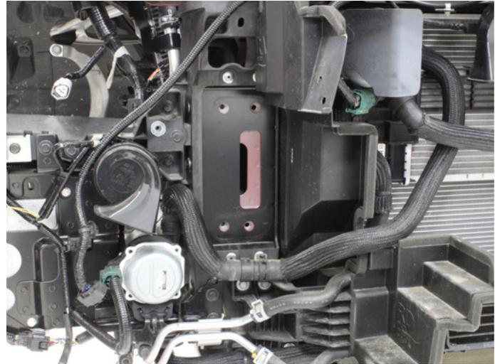
19. If equipped with an engine oil cooler, remove any plastic panels covering it.
