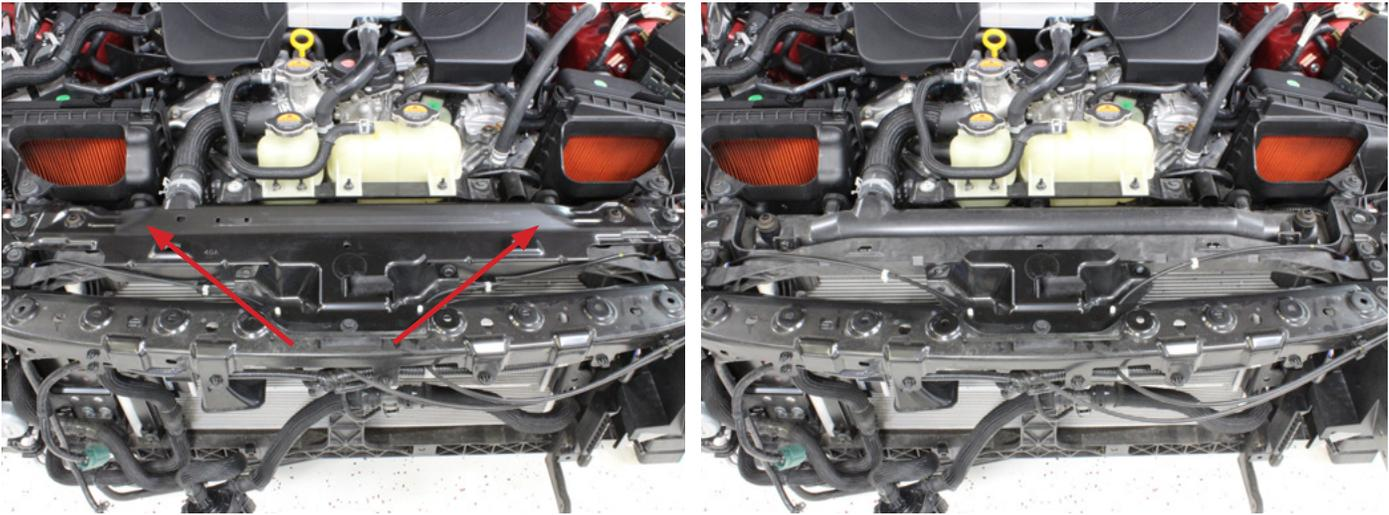
24. Drain the coolant out of the intercooler system only. The intercooler and engine coolant systems are separated. Remove the radiator cap from the small reservoir on the right side of the car. The system drain is on the bottom right side under the core support just under the main intercooler coolant pump.
