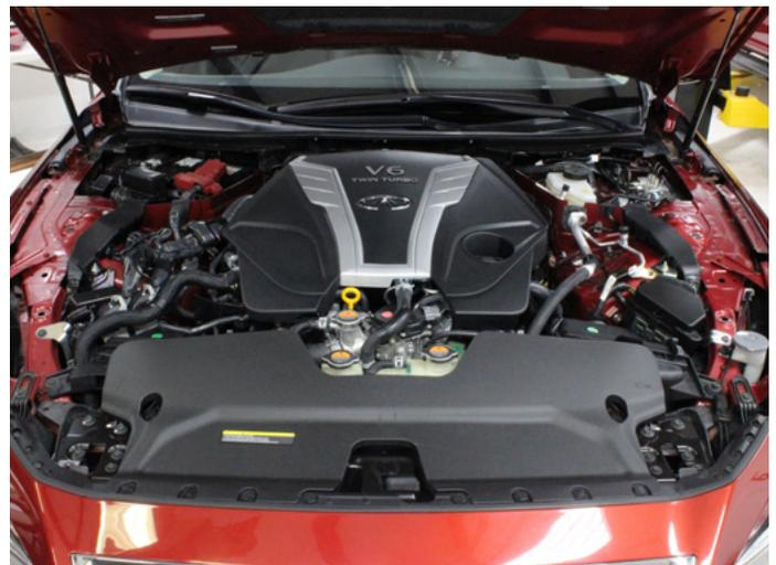
03. Remove the front core support cover / air box inlet duct panel.
