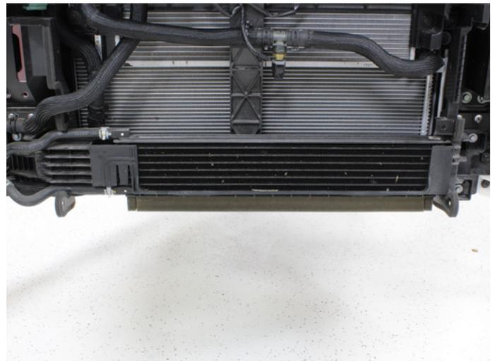
20. Remove the oil cooler. You do not need to disconnect the hoses. Remove the one bolt holding the metal lines in place on the right side and then remove the six bolts, three on each side. Allow the oil cooler to hang down.
