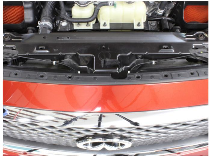
12. Carefully remove the front bumper. A second person is recommended for help. Make sure to pull the areas of the front bumper that meet the fender away from the headlights when removing. Painters tape is also highly recommended to protect any edges, panels, and headlights from being scratched during removal.
