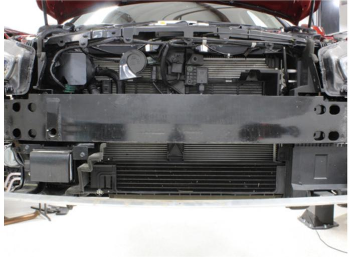
14. For the Q50 and Q60 if equipped, disconnect and remove the ICC (Radar Sensor) harness. The Q50 sensor is located in the lower right corner of the crash beam (shown). The Q60 is located on the top center of the crash beam.
