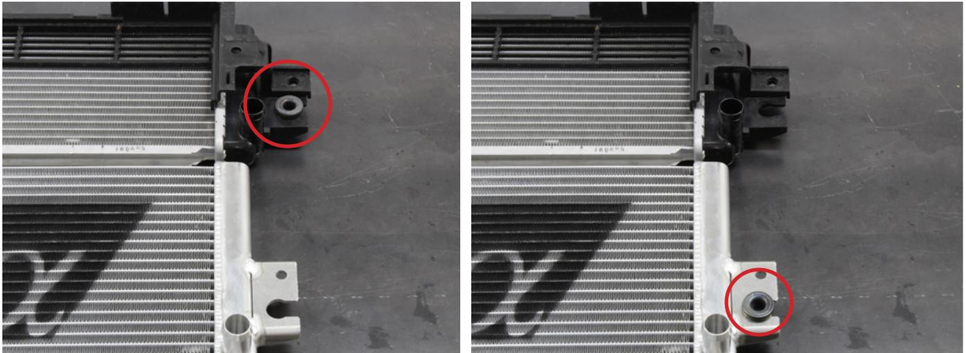
30. Locate the supplied foam stripping. Cut the material in half into two separate parts. Apply the foam stripping to the rear of the Infiniti Red Alpha heat exchanger along the weld seam.
