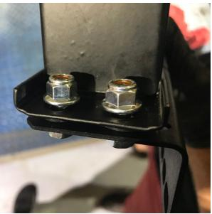
15. Attach the upper bracket to the cooler cure with the two supplied 10mm bolts and lock nuts. At the same time take the small section of rubber edging and cut a slit down the middle and slot it into the small gap on the upper bracket.
