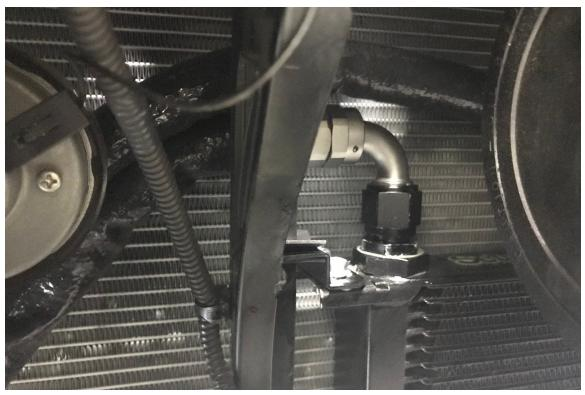
14. Attach the lower mounting bracket to the cooler core with the four supplied 10mm bolts and lock nuts **make sure to insert the bolts from the bottom to avoid clearance issues**. Use the 4 rubber washers in between the bracket and the cooler core to insulate the assembly.
