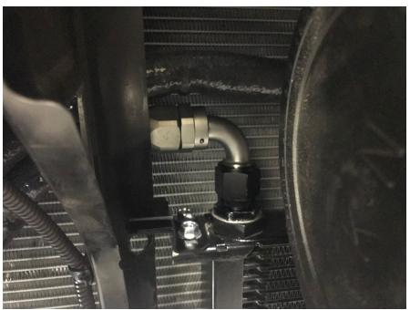
21. Now with the cooler in position, screw the two 10mm bottom mounting bolts into the barrel nuts installed in step #17.
