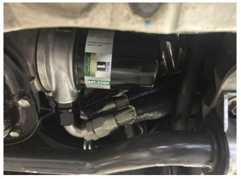
13. With one side of the lines hooked up, take the other side of the lines and wrap them over the front impact bar and in between the radiator/condenser and the vertical center brace for the front core support, where the top of the cooler core will mount.
