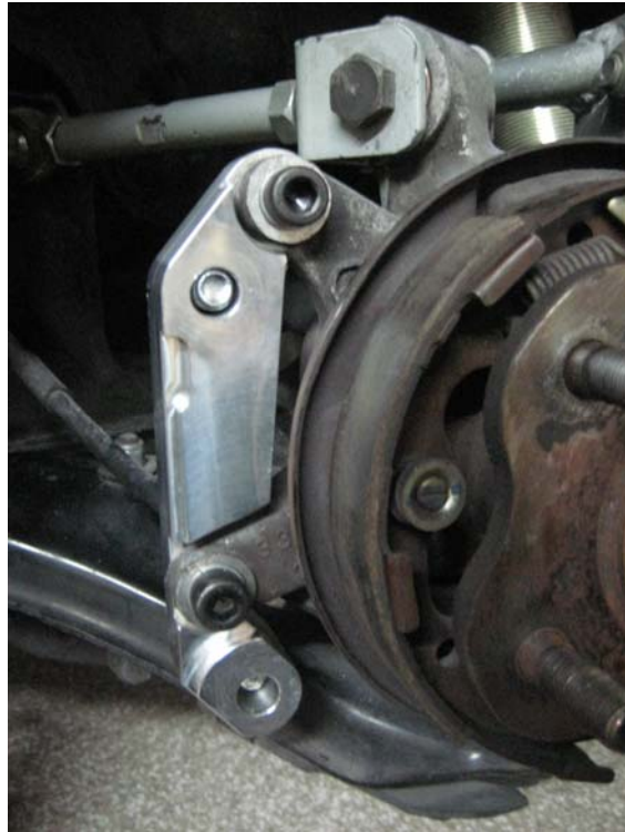
Figure 7: Bracket installed on hub
