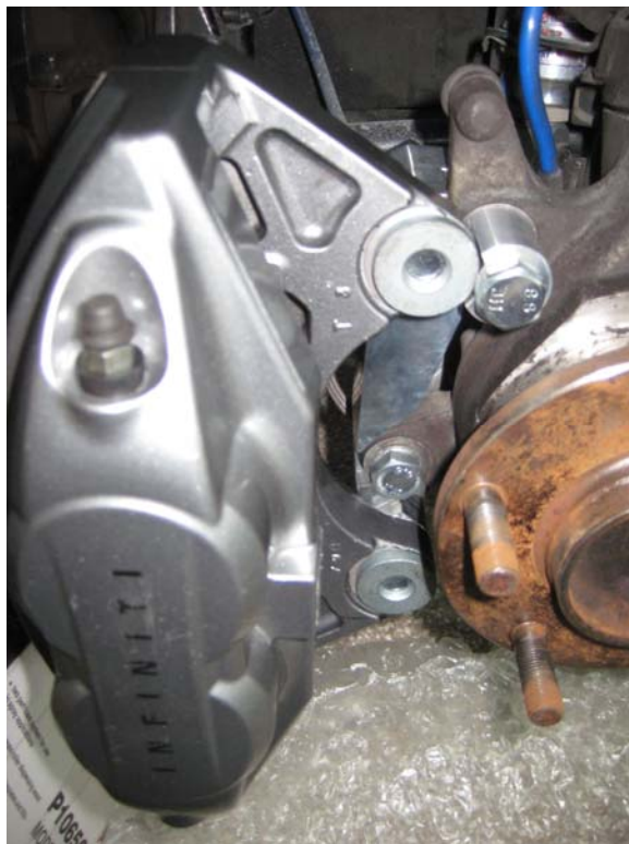
Figure 4: Assembly bolted to spindle
