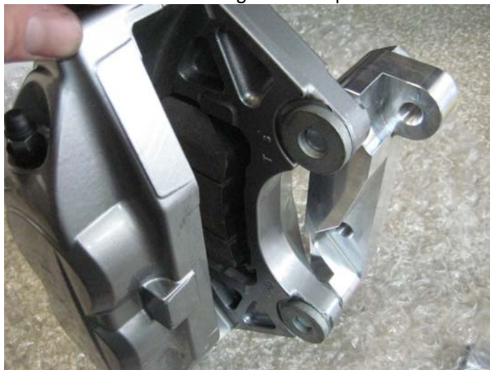
Figure 3: Driver's side bracket installed on caliper.
