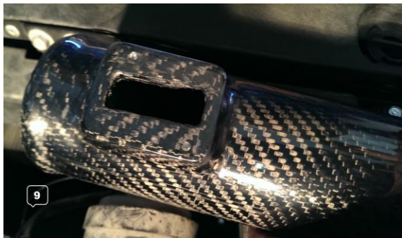
9. Need to Pre Align the Stock MAF Sensor to the CF Pipe Sensor Opening, Than required to drilled the Fitting Holes by 1/8" Drill Bits
