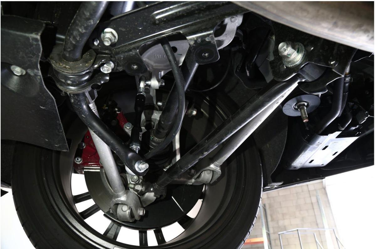
8. Tighten heim joint jam nuts against the center hex body of the sway bar endlink to **20-30 ft-lbs.**
