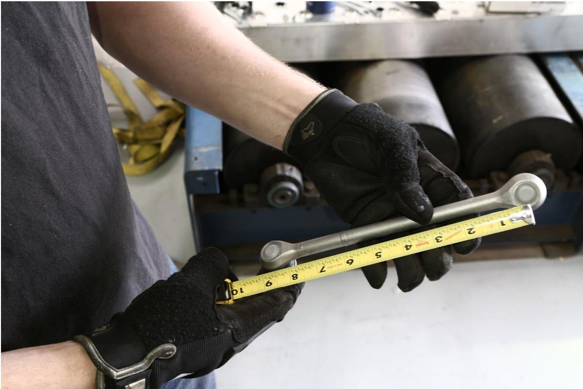
If the car is lowered, it is best to set the length with no preload. To do this, leave one link connected, and on the other side, install the link on just the spindle, leaving it disconnected from the sway bar. Set the car on the ground (all 4 wheels), and adjust the loose endlink until it easily installs in the sway bar. This will be your length setting for both sides. Ideally, the sway bar should be parallel to the ground once this is set.
