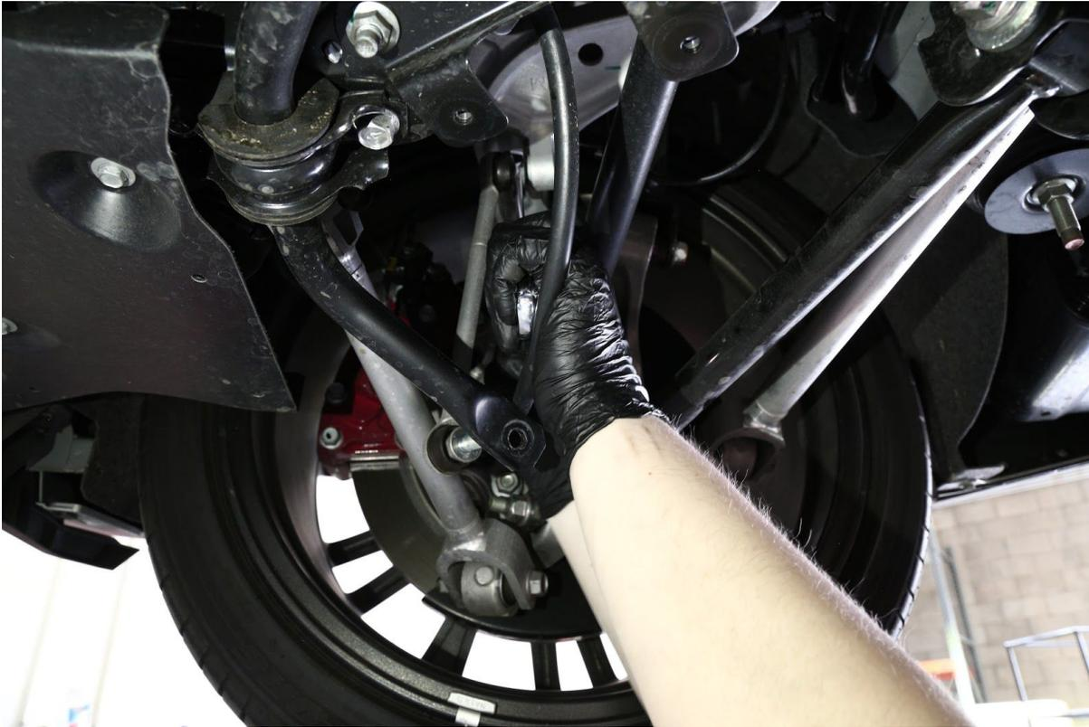
4. After removing, we need to set the length of the endlink. If the car is factory height, measure the distance between the center points on the two studs on the factory link, then adjust the SPL endlink to match. Match up the angle of the two end link studs as well, but don't tighten down the jam nuts yet.
