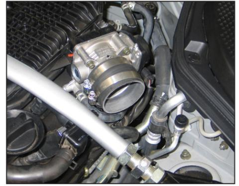
54. Install silicone hose (#08440) onto the throttle body and secure with the provided hose clamp.
