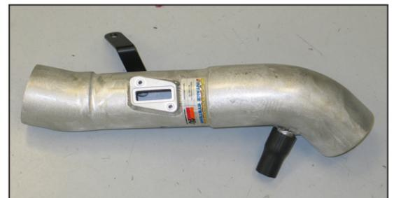
22. Install the provided 5/8" ID hose onto the vent fitting as shown.
