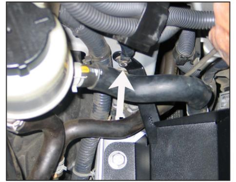
20. Secure the heat shield mounting bracket and ground strap with the provided hardware.
