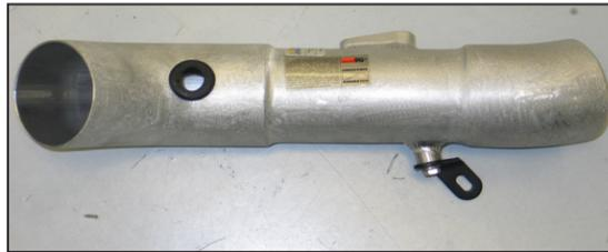
48. Install the provided rubber grommet into the K&N® intake tube as shown.
