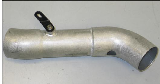
47. Install tube mounting bracket (#26665) onto the K&N® intake tube (#27540) with the provided hardware as shown.
