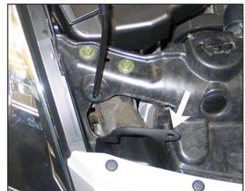
5. Remove the passenger side fresh air duct retaining clip. Slide the fresh air duct forward to disengage it from the passenger side airbox.
