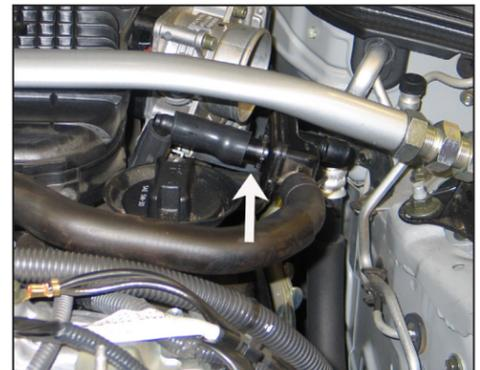
53. Connect the crankcase vent chamber into the 90° vent fitting assembly (installed in step #52).
