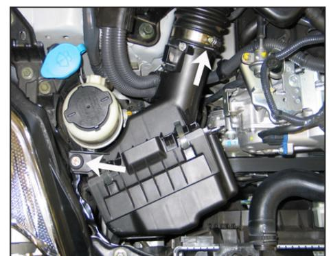
6. Loosen the hose clamp that secures the passenger side intake tube to the airbox. Then, remove the bolt that secures the passenger side airbox to the inner fender.
