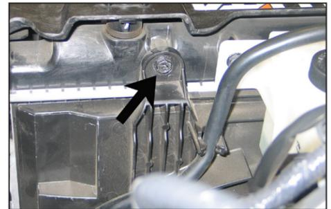
36. Remove the radiator cooling fan mounting bolt (shown).
