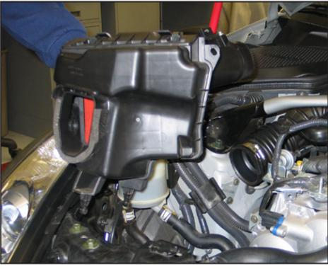
7. Remove the passenger side airbox as shown.
