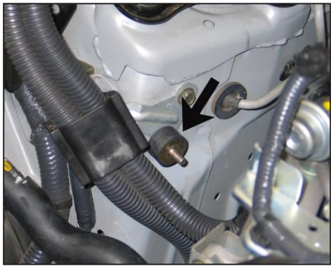
14. Install the provided rubber mounted stud into the battery cable mounting bracket bolt location (from step #13).
