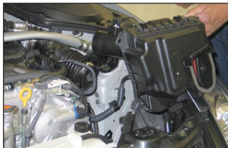
33. Remove the driver's side airbox as shown.
