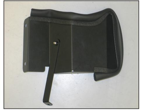
18. Install the heat shield mounting bracket (#26663) onto the heat shield with the provided hardware as shown.
