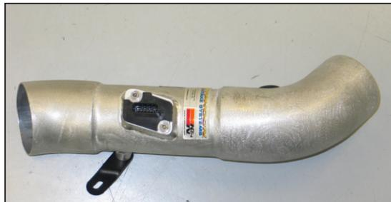
50. Install the mass air sensor into the K&N® intake tube (#27540) and secure with the provided hardware.
