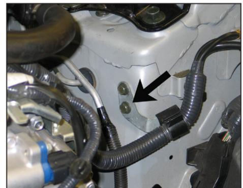
40. Remove the lower ground strap mounting bracket bolt shown.
