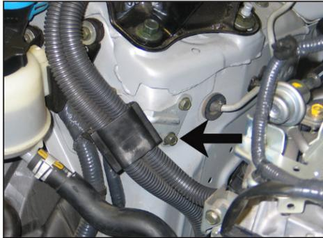
13. Remove the lower battery cable mounting bracket bolt shown.
