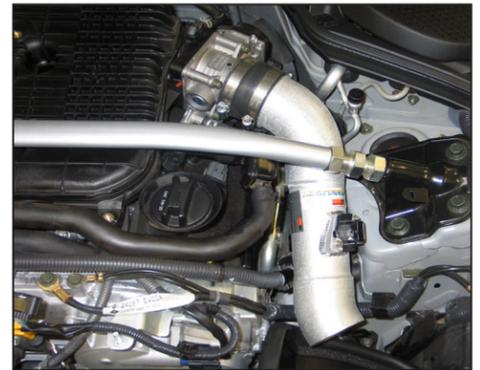
55. Install the intake tube assembly into the silicone hose at the throttle body and align the mounting bracket with the rubber mounted stud (installed in step #41). Insert the crankcase vent chamber into the grommet in the intake tube. Secure the intake tube with the provided hardware and hose clamp. **NOTE: Ensure the crankcase vent chamber has a good seal in the grommet installed into the intake tube.**
