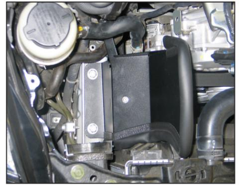
19. Install the heat shield assembly into the engine compartment and align it with the inserted nuts (installed in step #16). Secure the heat shield to the inserted nuts with the provided hardware.
