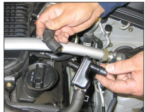
39. Disconnect the crankcase vent chamber hose from the engine valve cover, then from the crankcase vent chamber as shown.
