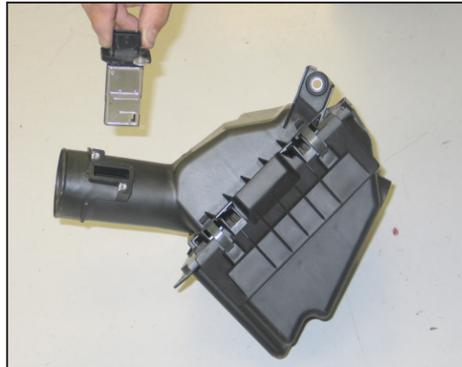
49. Remove the mass air sensor from the factory airbox as shown.
