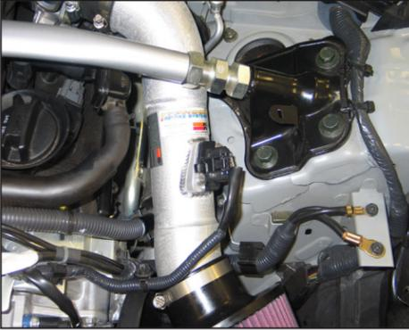
57. Re-connect the mass air sensor electrical connection.
