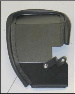
44. Install the provided lower heat shield mounting bracket (#06488) onto the bottom of the heat shield and secure using the provided hardware and spacer (as shown).
