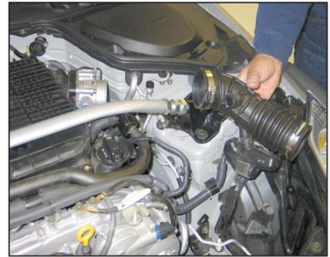
38. Release the spring clamp that secures the crankcase vent chamber to the intake tube. Then, remove the driver's side intake tube as shown.
