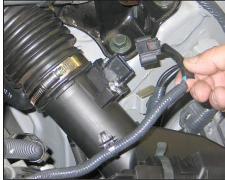
30. Unhook the driver's side mass air sensor wiring harness from the airbox, then disconnect the mass air sensor electrical connection as shown.
