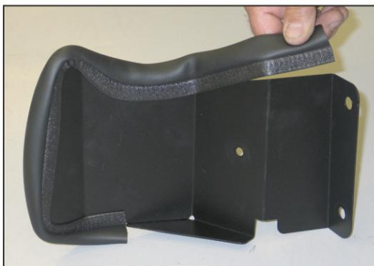
17. Install the provided edge trim onto the heat shield (#07366) as shown.
