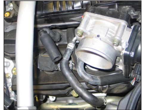
52. Install the 90° crankcase vent fitting assembly onto the valve cover as shown.
