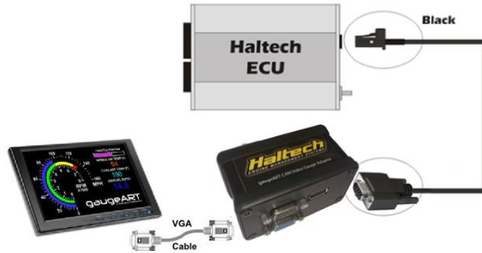
Figure 3 – Haltech GaugeART CAN Video Gauge Adapter connected directly to a Haltech Platinum Series ECU
