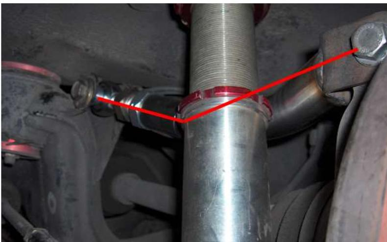
There is a small angle designed into the arm to allow it more clearance to the frame rail for lowered cars. If installed in the wrong orientation there will be LESS clearance to the frame rail than normal, and can result in damage or failure of the rear upper arms. Properly installed, the angle would be as shown.
