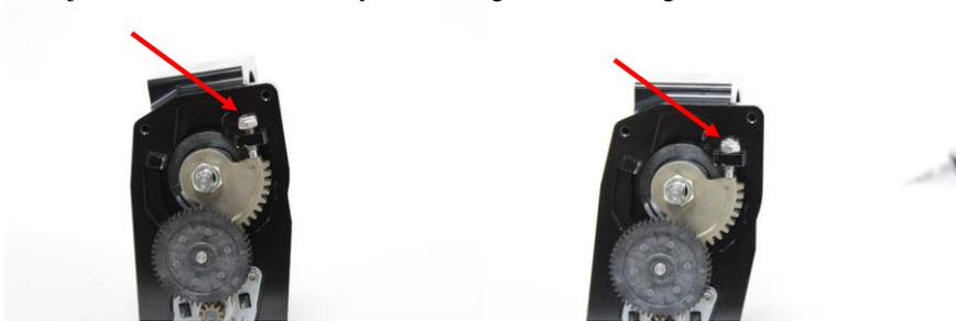
21) Now install the resting position set screw. This screw sets the resting throttle plate position. **Important: The final position of this screw must be set by your tuner.** To get a baseline, turn the screw in until it touches the stop cam or you feel the throttle plate just start to move from fully closed. Then Turn the screw 2 full revolutions clock-wise. Lock the screw down with the lock nut.
