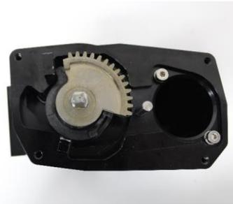
14) Install the drive motor using the two screws provided.
