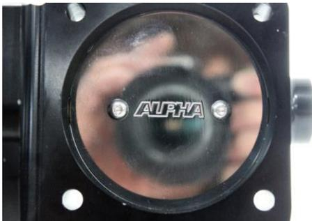
**19)** Install the smaller set screw into the location shown. This set screw is used to set fully closed position of the throttle plate.
