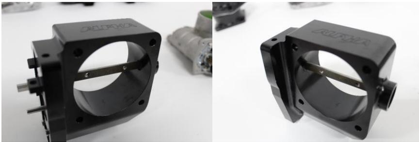
13) Install the throttle shaft gear and spring. Note the following pictures for orientation and position of the spring. The spring must sit in the detents shown in the pictures with the arrows.
