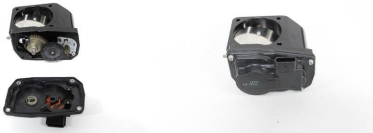
23) Install the Alpha endcap. Use green sleeve retaining compound on the mating edge of the endcap. Align and drive into place with a plastic or soft mallet.
