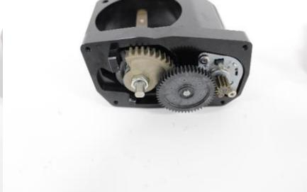
16) Insert the throttle plate into the throttle body housing. Make sure the throttle plate and housing are both facing a direction in which "ALPHA" can be read.
