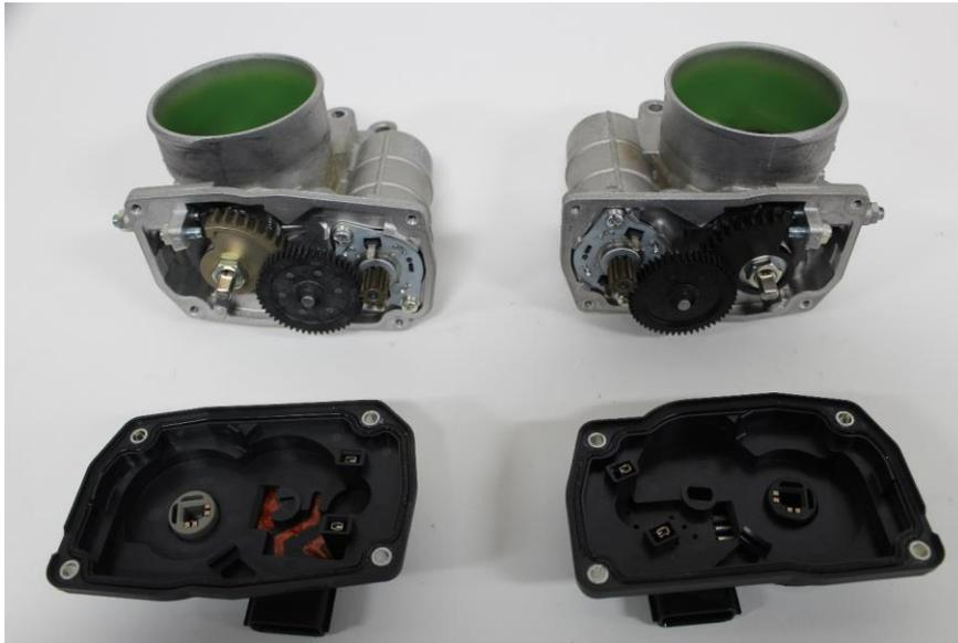
4) **Note:** When removing the covers, it's possible for the electrical connector to pull out from the cover and stay attached to the drive motor. Don't worry, just remove the connector from motor carefully, and reinsert into the cover with light pressure to seat it all the way down.
