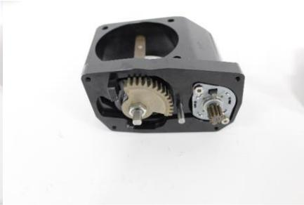
15) Install the intermediate gear.
