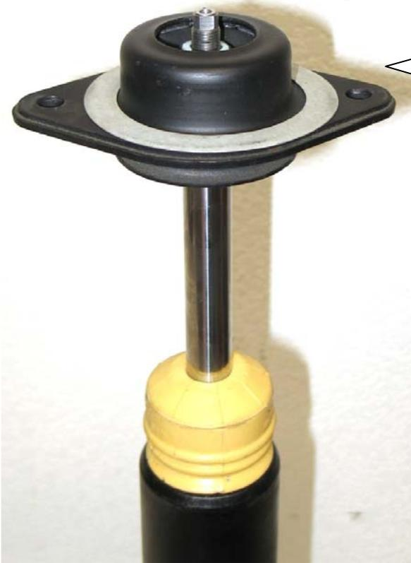
Install the factory supporting bearing and fix it with the supplied nuts. Tightening torque for the piston rod nut is 20 Nm (15 ft-lb). The damper unit has to be installed according to manufacturers recommended settings regarding tightening torque and fixing specifications.
