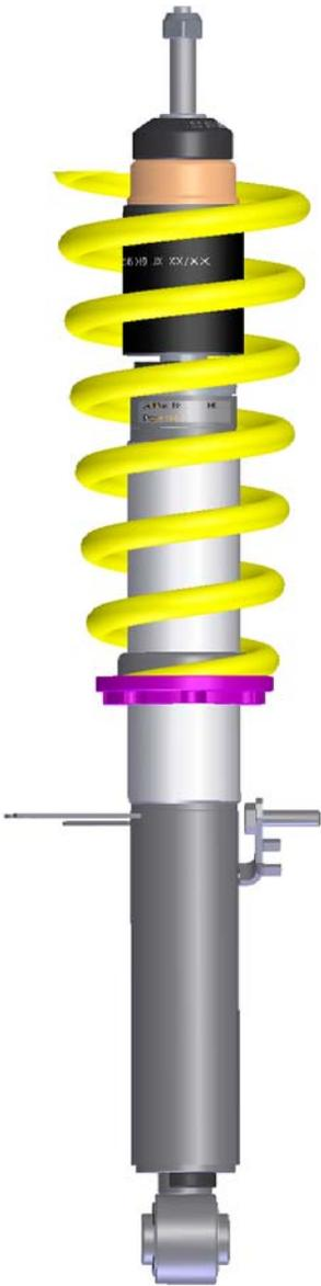
Install the factory supporting bearing without the standard bump stop and fix it with the supplied stop nut. Tightening torque for the piston rod nut is 35 Nm (26 ft-lb). The strut unit has to be installed according to manufacturers recommended settings regarding tightening torque and fixing specifications.
