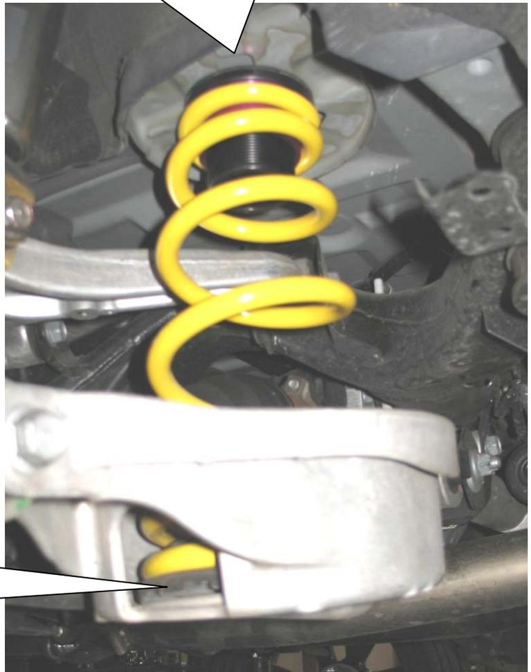
Use the original spring support at the bottom end of the spring.
