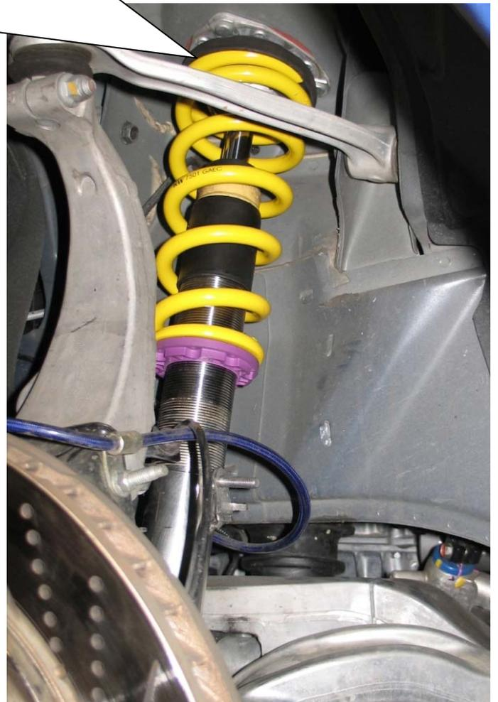
After you have completed installation of the suspension, check the clearance of the tyres to the front suspension strut. The minimum clearance at the narrowest point is 5 mm and must, where necessary, be provided using commercially available, Technical Inspectorate (German TÜEV) approved spacers.
