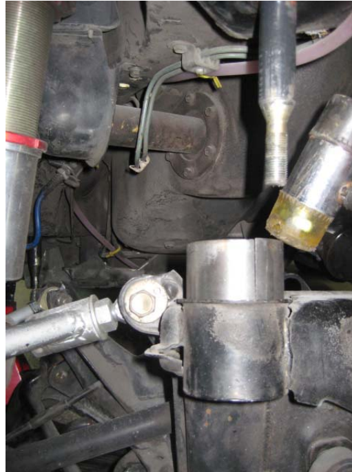
Installing bushing shell
