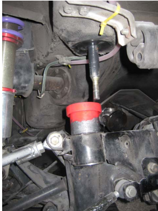
Bushing with light coating of grease
