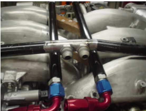
Figure 2 — Modified balance/crossover tube
