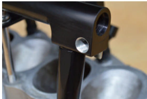
Figure 13 – Fuel temperature sensor boss
