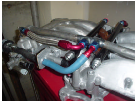
Figure 3 — Idle air plumbed with AN hose fittings
