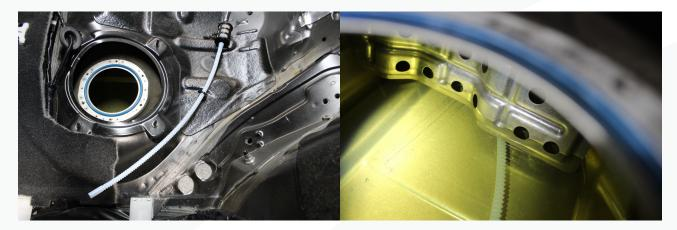
44. Push the open end of the hose onto the metal tube at the front of the tank.
