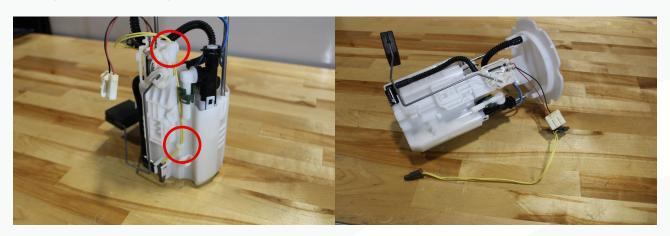
14. Push the level sensor retaining lock over and slide the sensor up and out.
