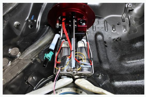
57. Connect the black hose to the hose installed in the previous step. Then connect the New siphon pickup hose to the fitting on the right side.
