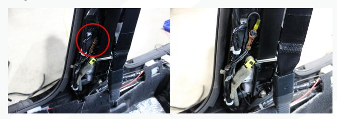
80. Stretch out the 3/8" split loom from the relay towards the front of the car and up into the dash area, mark it, then add 24" so it reaches into the battery compartment.
