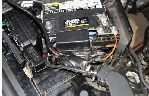
89. This completes the installation of the AMS Single Pump LSFP. Check over your work and install the fuses. Make sure to check for leaks before reassembling the vehicle.
