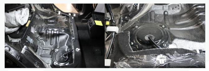
6. Remove the access panel and disconnect the fuel line quick disconnect and top hat electrical connector.
