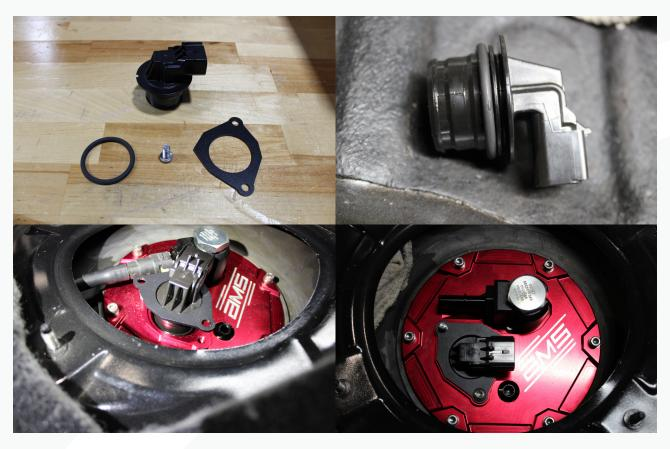
61. Install the white quick disconnect clip removed earlier onto the top hat fitting. Reconnect the factory fuel line.
