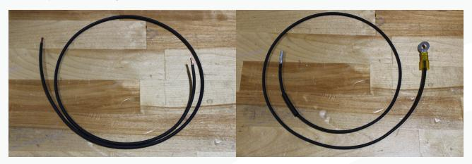
77. Crimp the wire from the previous step to the wire you stripped from the 2-pin connector. Slide over the heat shrink and use a heat gun to shrink the heat shrink over the butt connector and the ring terminal.
