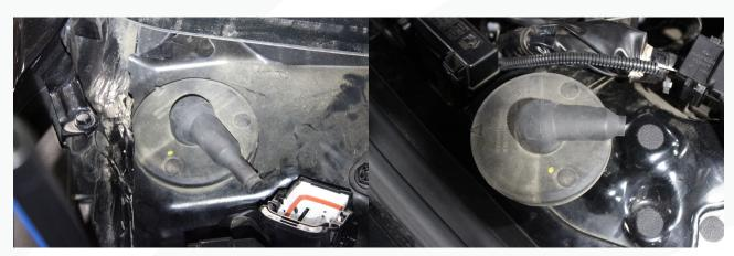
85. Feed the wires up through the hole into the battery compartment. Then while holding the grommet, feed the wires and loom through the grommet at click the grommet back in place.
