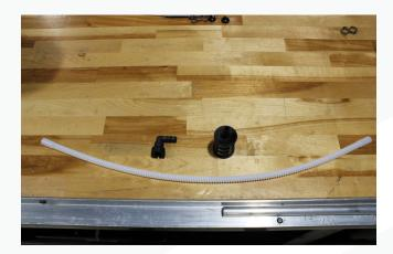
40. Assemble the hose as shown below, using the cinch clamp on the siphon strainer. Again, using a small amount of heat without damaging the hose, affix the 3/8 quick connect fitting to the other end of the siphon hose. Measure 6" from the strainer, fix the magnet to the hose with 1 zip tie.
