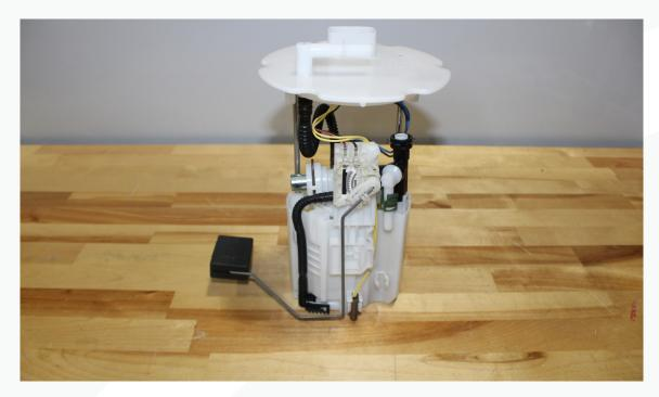
12. Disconnect the two electrical connectors.
