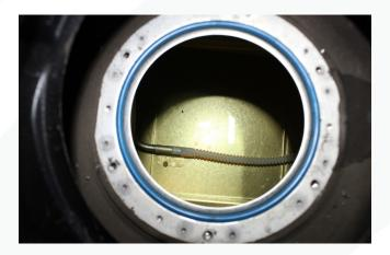
45. Reinstall the driver's side top hat and replace the O-ring if necessary. Then reinstall the connector and cover panel.
