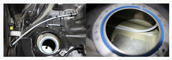
47. Install the short siphon hose into the black hose connection inside the tank.
