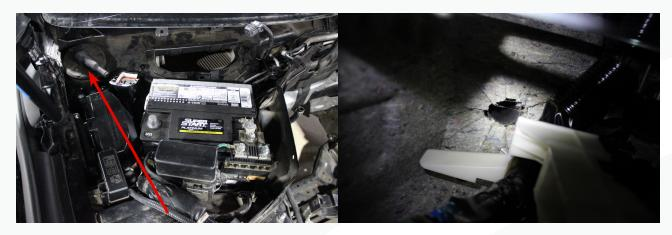
84. Trim the grommet just before it enlarges. This spot will fit tight on the loom to help prevent leaks.
