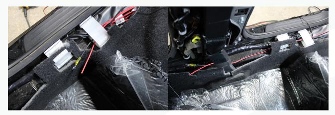
79. Locate the chassis ground on the b pillar above the seat belt retractor and install the ring terminal.
