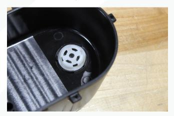
36. On the side of the basket there will be two dimple features. The Q50/60 you will need to drill the top hole with a 13/64 drill bit. On the Z the basket has three tiers, so you will need to drill both the holes on the middle tier only!
