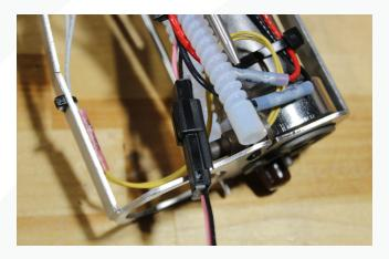
31. Cut off the OEM level sensor connector about an inch away from the connector.
