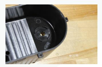
35. Carefully place the flapper door retainer over the flapper being careful not to damage it. Be sure the retainer is fully secured into the basket. Tip the basket over to be sure the flapper door can move freely.
