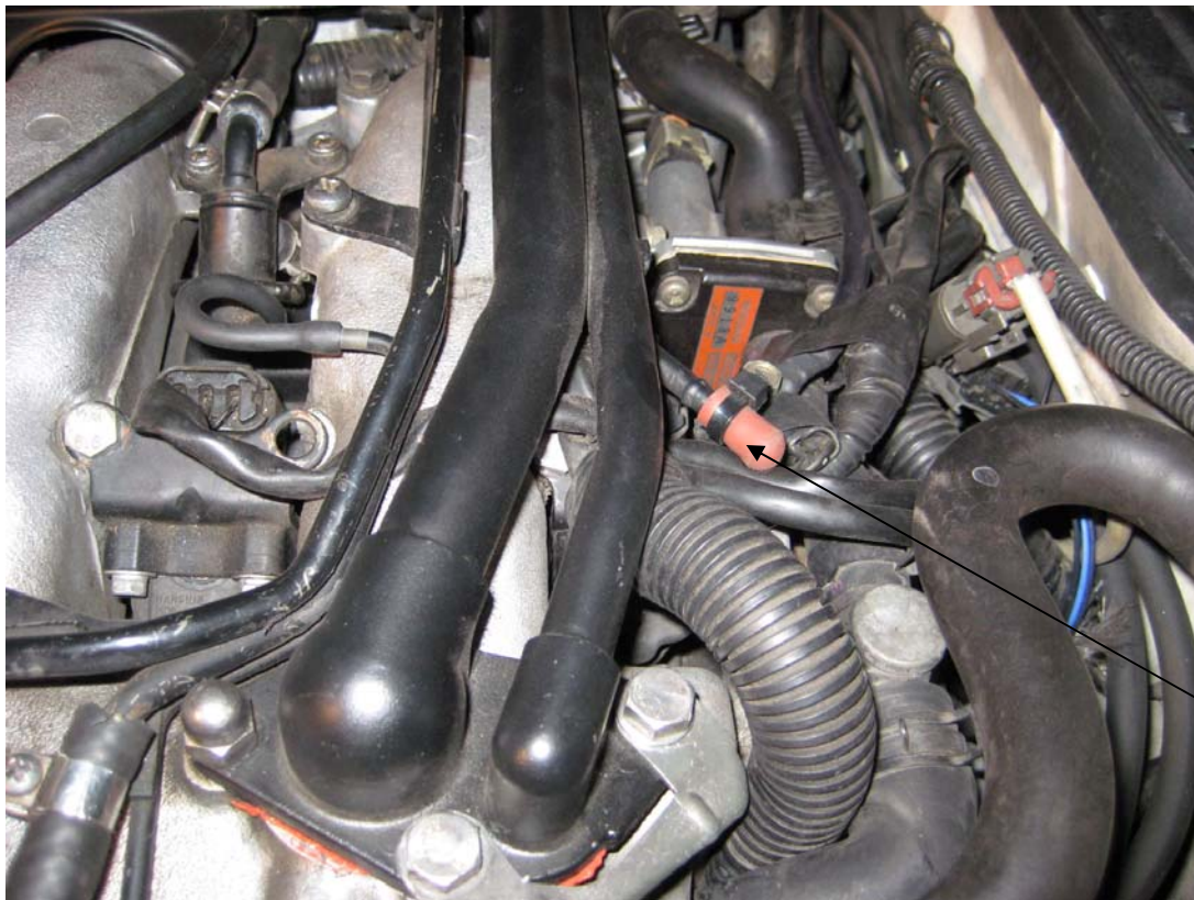
Plug port on driver's side of plenum balance tube
